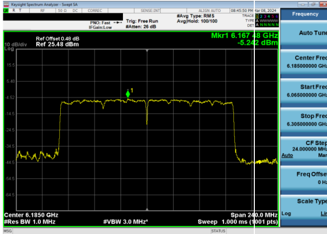
Plot 7-383. SP Power Spectral Density Plot CDD Diversity Antenna WF2a (160MHz 802.11ax RU996x2 (UNII Band 5) – Ch. 47)
