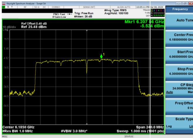
Plot 7-384. SP Power Spectral Density Plot CDD Diversity Antenna WF7b (160MHz 802.11ax RU996x2 (UNII Band 5) – Ch. 47)
