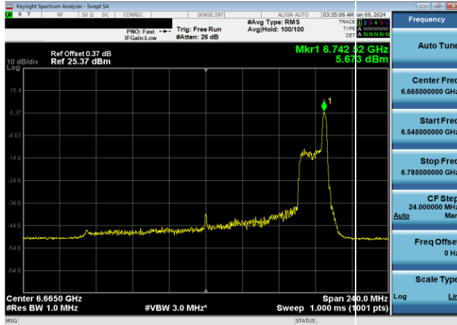
Plot 7-413. SP Power Spectral Density Plot CDD Diversity Antenna WF2a (160MHz 802.11ax RU26 (UNII Band 7) – Ch. 143)
