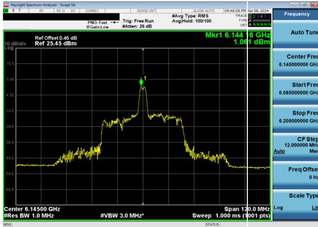
Plot 7-372. SP Power Spectral Density Plot CDD Diversity Antenna WF7b (80MHz 802.11ax RU26 (UNII Band 5) – Ch. 39)
