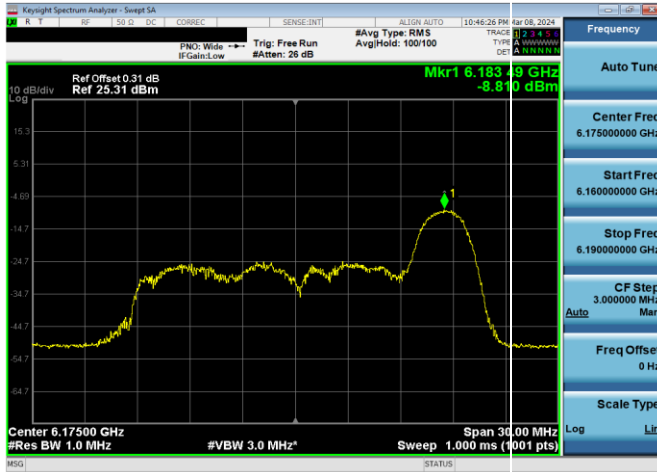
Plot 7-419. LPI Power Spectral Density Plot Antenna WF7a (20MHz 802.11ax RU26 (UNII Band 5) – Ch. 45)
