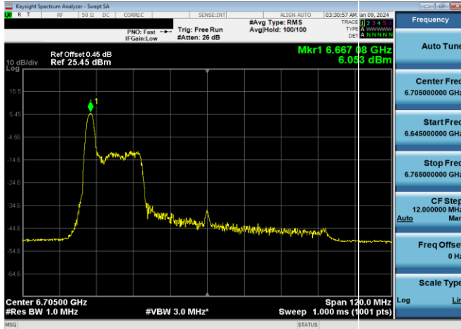
Plot 7-401. SP Power Spectral Density Plot CDD Diversity Antenna WF2a (80MHz 802.11ax RU26 (UNII Band 7) – Ch. 151)
