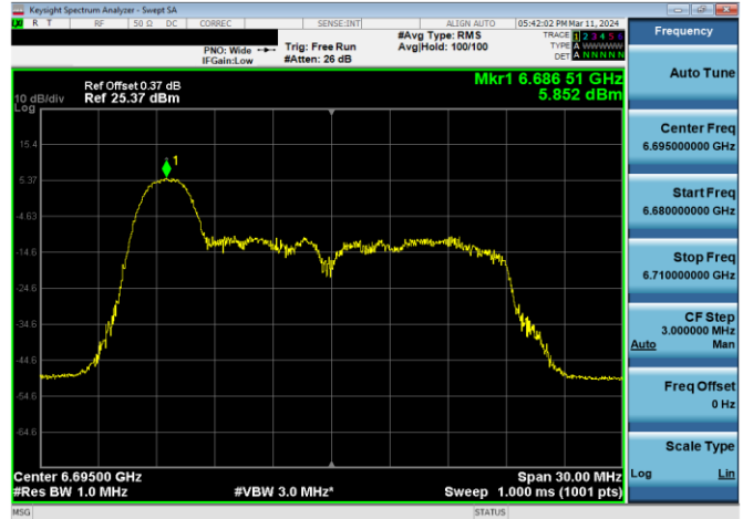
Plot 7-386. SP Power Spectral Density Plot CDD Diversity Antenna WF7b (20MHz 802.11ax RU26 (UNII Band 7) – Ch. 149)
