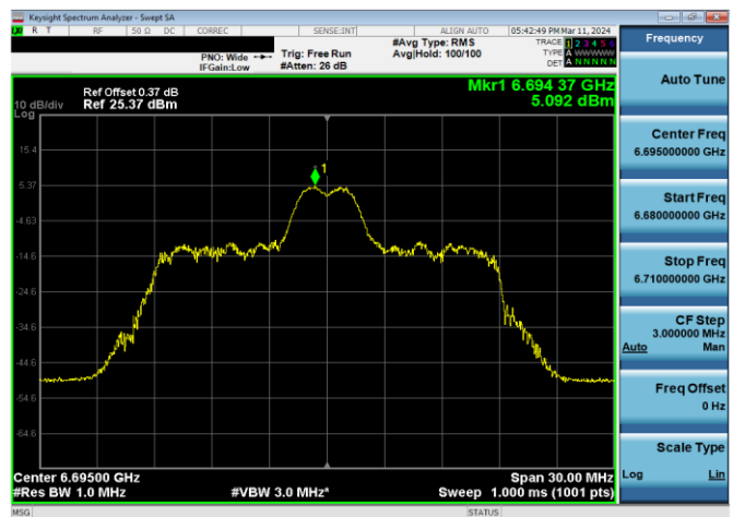
Plot 7-388. SP Power Spectral Density Plot CDD Diversity Antenna WF7b (20MHz 802.11ax RU26 (UNII Band 7) – Ch. 149)
