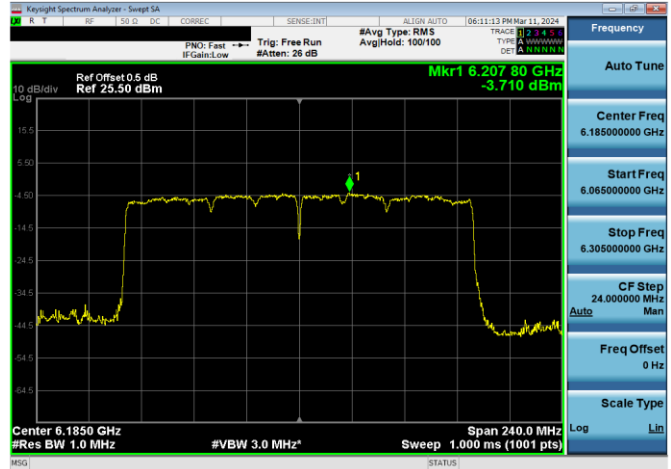
Plot 7-432. LPI Power Spectral Density Plot Antenna WF7a (160MHz 802.11ax RU996x2 (UNII Band 5) – Ch. 47)
