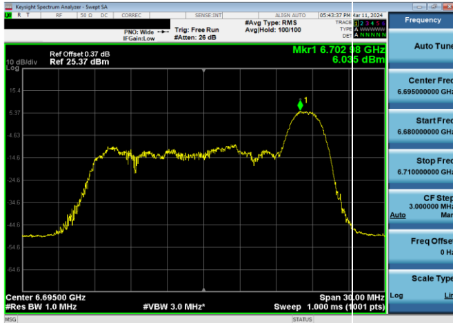
Plot 7-390. SP Power Spectral Density Plot CDD Diversity Antenna WF7b (20MHz 802.11ax RU26 (UNII Band 7) – Ch. 149)
