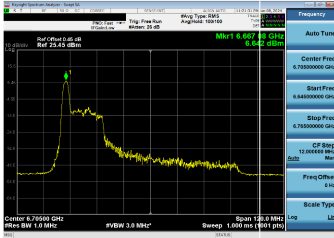
Plot 7-337. SP Power Spectral Density Plot CDD Primary Antenna WF7a (80MHz 802.11ax RU26 (UNII Band 7) – Ch. 151)
