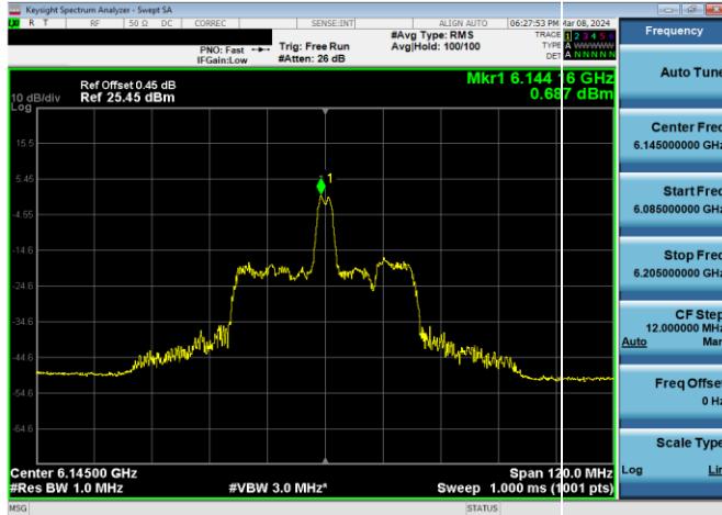
Plot 7-307. SP Power Spectral Density Plot CDD Primary Antenna WF7a (80MHz 802.11ax RU26 (UNII Band 5) – Ch. 39)
