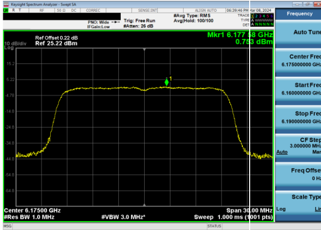
Plot 7-295. SP Power Spectral Density Plot CDD Primary Antenna WF7a (20MHz 802.11ax RU242 (UNII Band 5) – Ch. 45)
