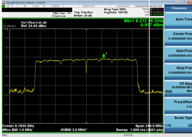
Plot 7-319. SP Power Spectral Density Plot CDD Primary Antenna WF7a (160MHz 802.11ax RU996x2 (UNII Band 5) – Ch. 47)
