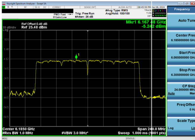
Plot 7-320. SP Power Spectral Density Plot CDD Primary Antenna WF2a (160MHz 802.11ax RU996x2 (UNII Band 5) – Ch. 47)
