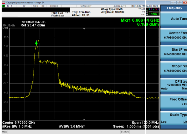
Plot 7-217. SP Power Spectral Density Plot Antenna WF7a (80MHz 802.11ax RU26 (UNII Band 7) – Ch. 151)
