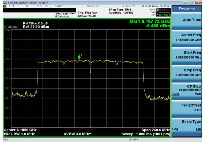
Plot 7-240. SP Power Spectral Density Plot Antenna WF2a (160MHz 802.11ax RU996x2 (UNII Band 5) – Ch. 47)
