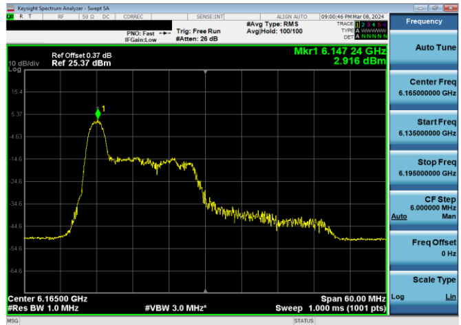
Plot 7-261. SP Power Spectral Density Plot Antenna WF7b (40MHz 802.11ax RU26 (UNII Band 5) – Ch. 43)
