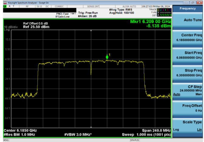
Plot 7-272. SP Power Spectral Density Plot Antenna WF7b (160MHz 802.11ax RU996x2 (UNII Band 5) – Ch. 47)
