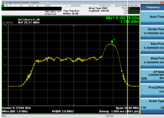
Plot 7-195. SP Power Spectral Density Plot Antenna WF7a (20MHz 802.11ax RU26 (UNII Band 5) – Ch. 45)
