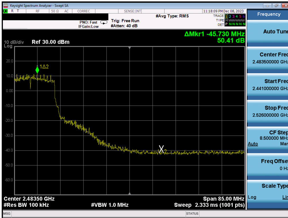
Plot 7-361. Band Edge Plot Antenna WF2b (802.11n (2.4GHz) – Ch. 8) – MCS4
