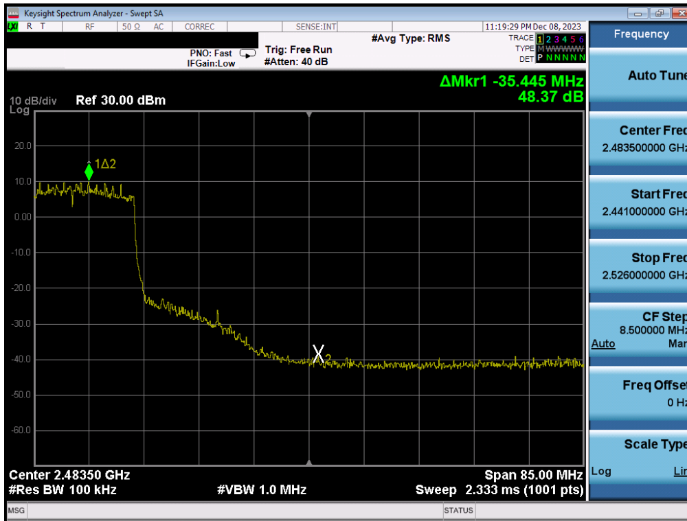
Plot 7-375. Band Edge Plot Antenna WF2b (802.11ax(SU) - (2.4GHz) – Ch. 8) – MCS4
