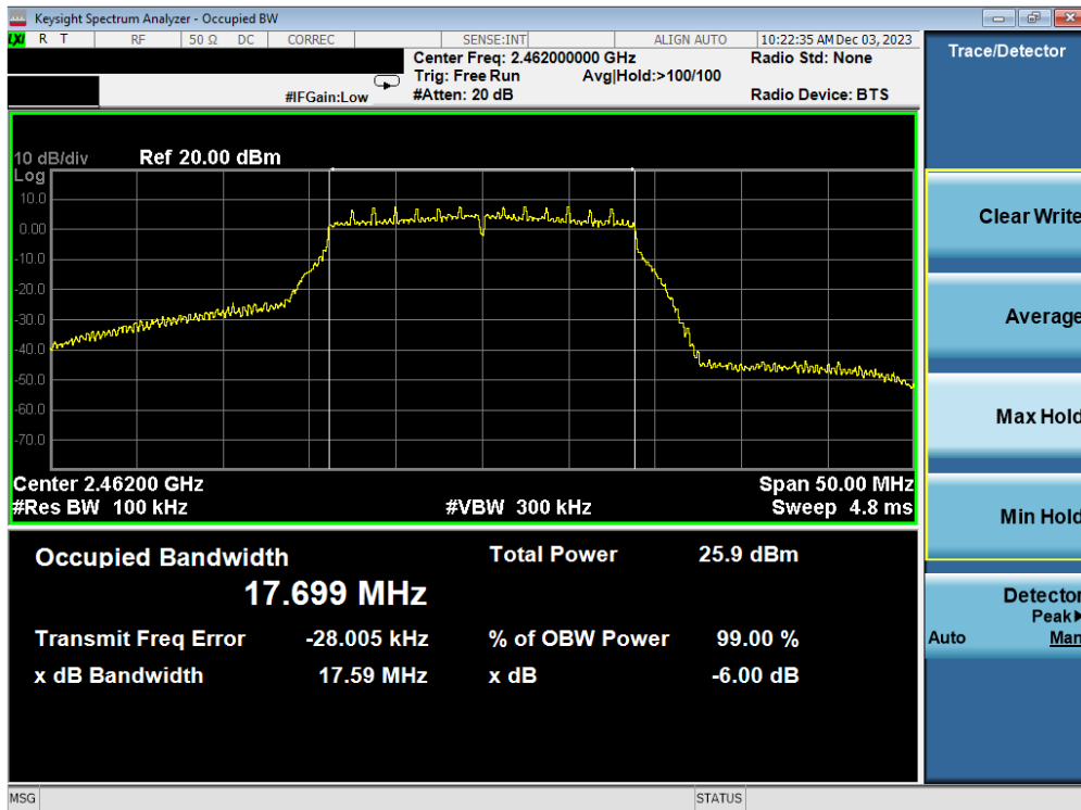
Plot 7-6. 6 dB BW and 99% OBW Plot Antenna WF7b (802.11n (2.4GHz) – Ch. 11) – MCS2
