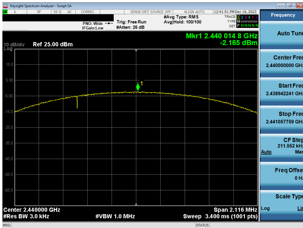
Plot 7-20. Power Spectral Density Plot Antenna WF7b (Bluetooth (LE), 2Mbps, ePA – Ch. 19)
