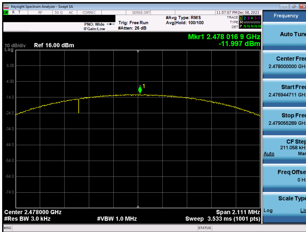
Plot 7-60. Power Spectral Density Plot Antenna WF2b (Bluetooth (LE), 2Mbps, iPA – Ch. 38)
