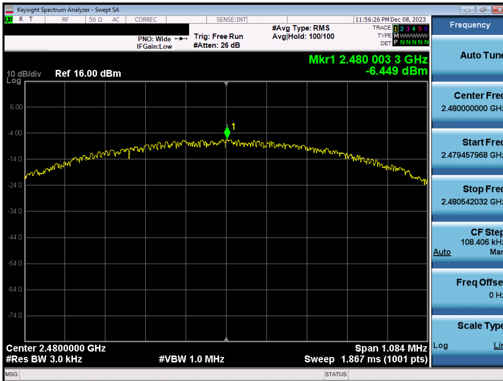
Plot 7-48. Power Spectral Density Plot Antenna WF2b (Bluetooth (LE), 1Mbps, iPA – Ch. 39)
