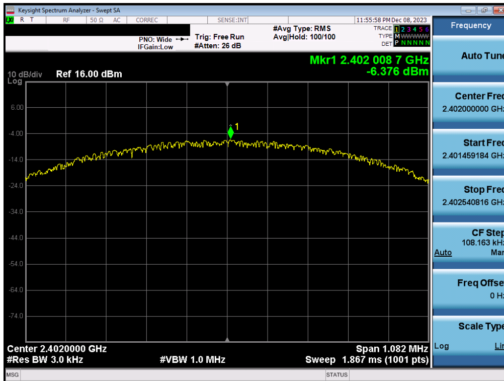
Plot 7-44. Power Spectral Density Plot Antenna WF2b (Bluetooth (LE), 1Mbps, iPA – Ch. 0)
