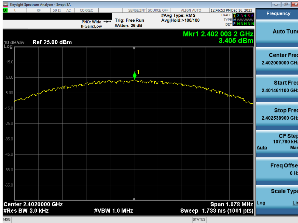
Plot 7-37. Power Spectral Density Plot Antenna WF7b (Bluetooth (LE), 1Mbps, ePA – Ch. 0)
