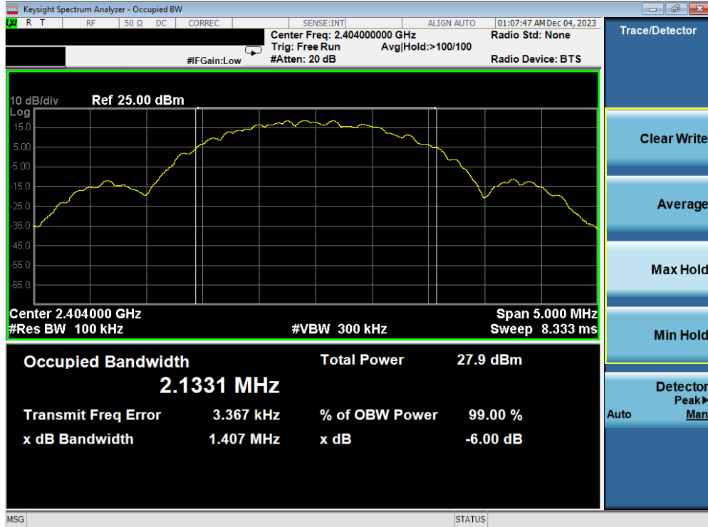
Plot 7-10. 6dB BW & 99% OBW Plot Antenna WF2b (Bluetooth (LE), 2Mbps, ePA – Ch. 1)
