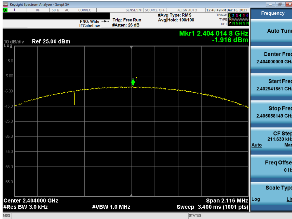
Plot 7-49. Power Spectral Density Plot Antenna WF7b (Bluetooth (LE), 2Mbps, ePA – Ch. 1)
