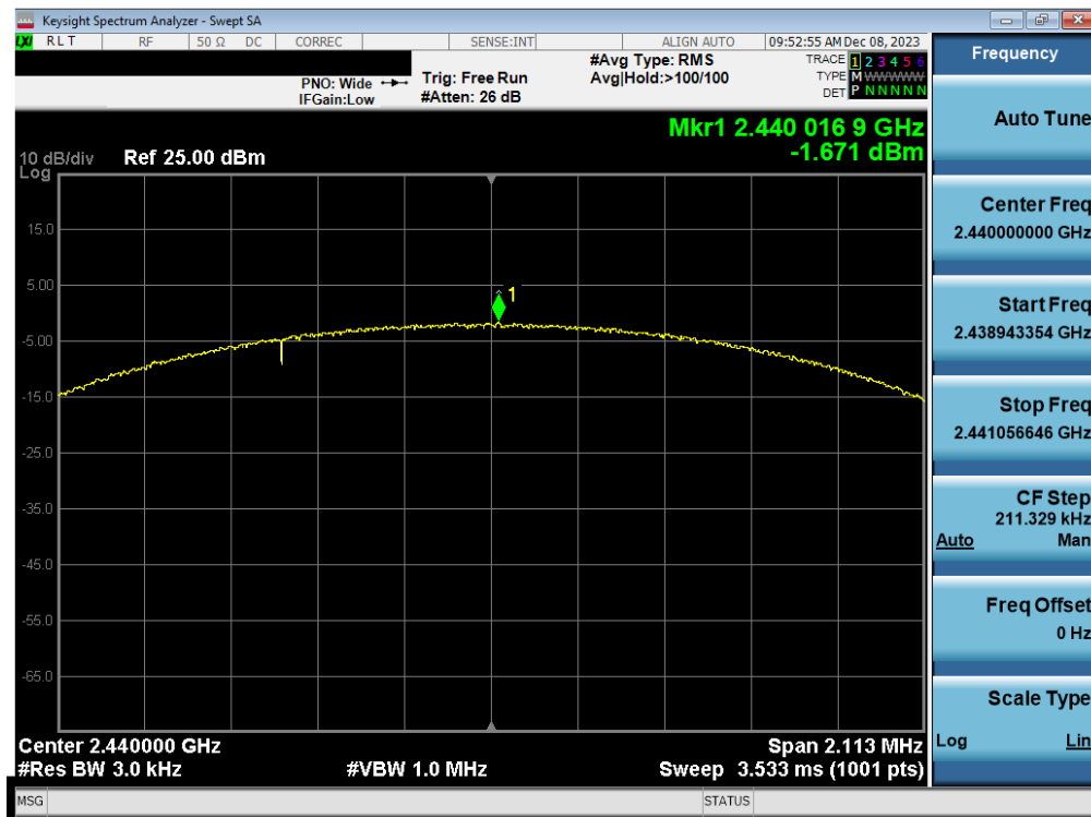
Plot 7-52. Power Spectral Density Plot Antenna WF2b (Bluetooth (LE), 2Mbps, ePA – Ch. 19)
