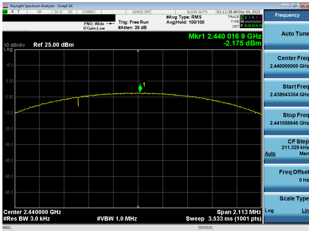
Plot 7-32. Power Spectral Density Plot Antenna WF2b (Bluetooth (LE), 2Mbps, ePA – Ch. 19)
