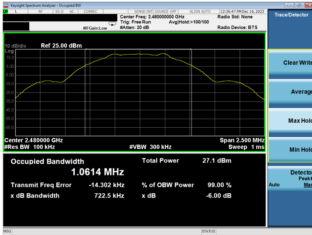
Plot 7-3. 6dB BW & 99% OBW Plot Antenna WF7b (Bluetooth (LE), 1Mbps, ePA – Ch. 39)
