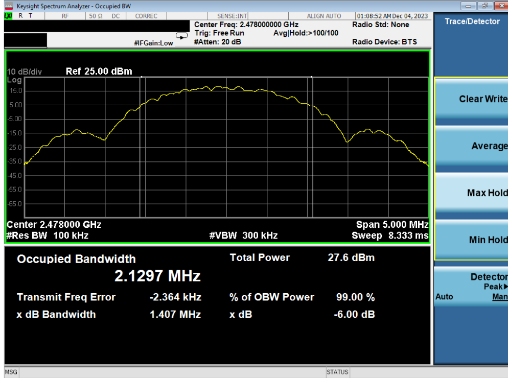
Plot 7-12. 6dB BW & 99% OBW Plot Antenna WF2b (Bluetooth (LE), 2Mbps, ePA – Ch. 38)
