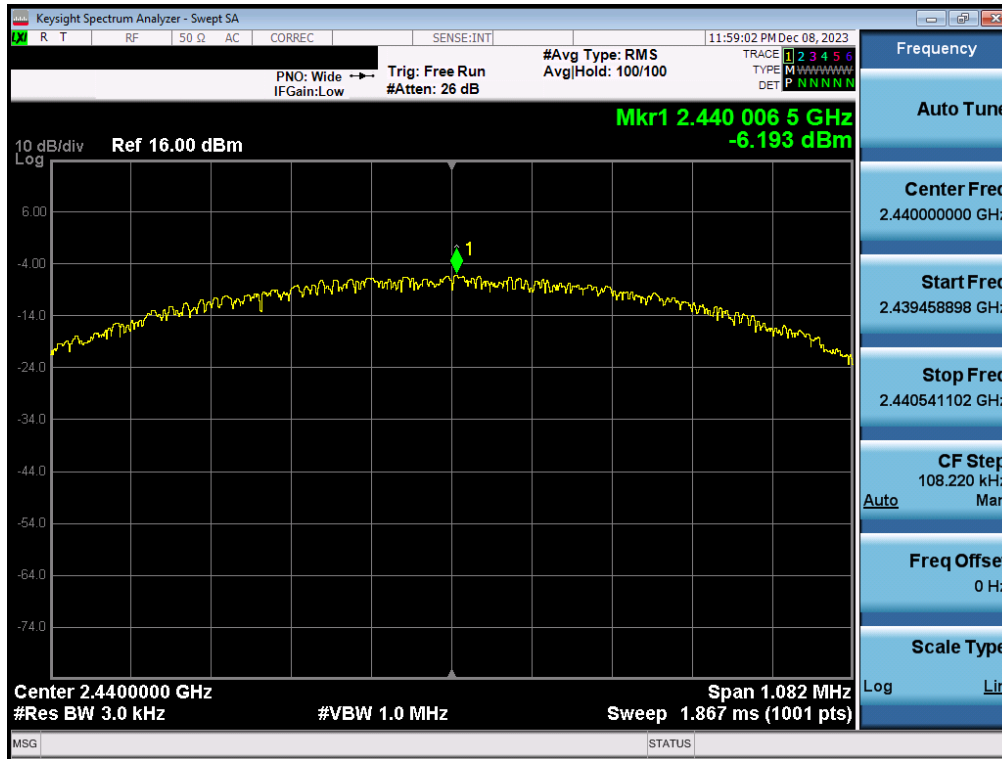
Plot 7-29. Power Spectral Density Plot Antenna WF2b (Bluetooth (LE), 1Mbps, iPA – Ch. 19)
