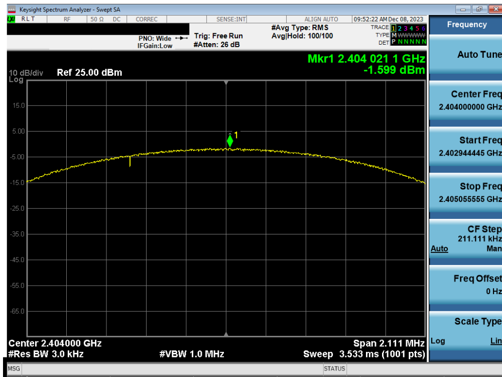
Plot 7-50. Power Spectral Density Plot Antenna WF2b (Bluetooth (LE), 2Mbps, ePA – Ch. 1)
