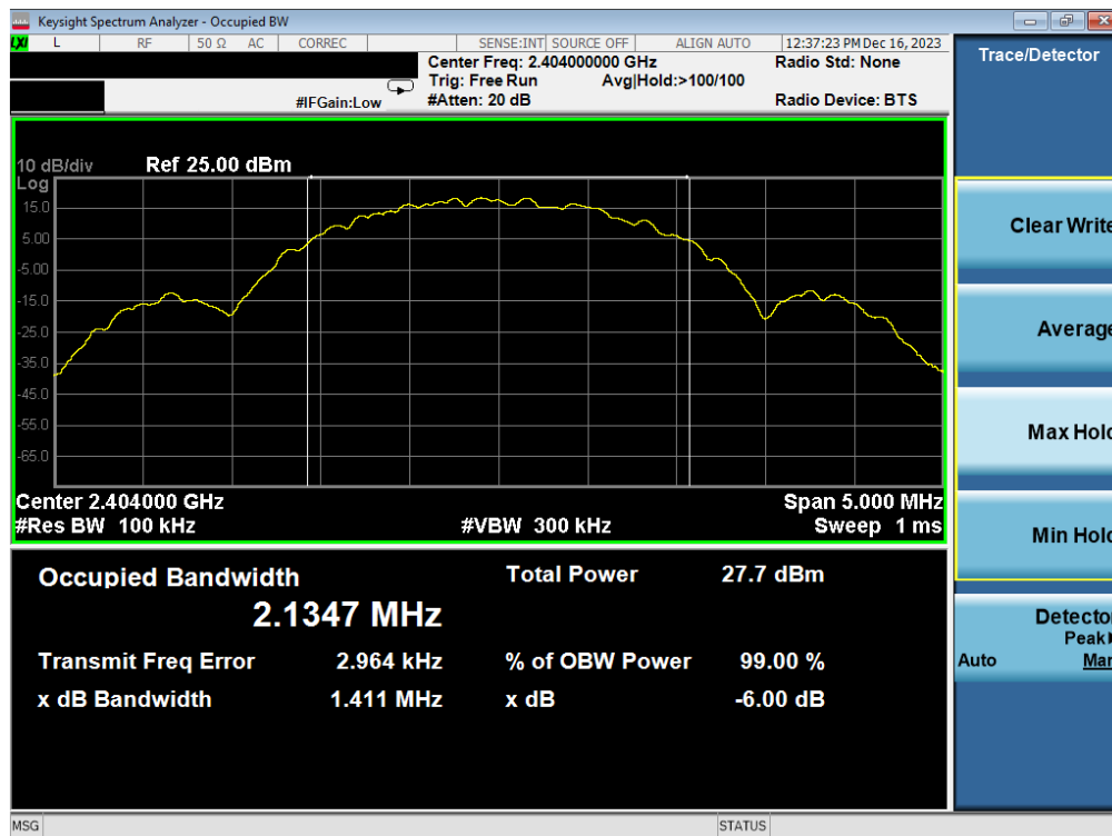
Plot 7-4. 6dB BW & 99% OBW Plot Antenna WF7b (Bluetooth (LE), 2Mbps, ePA – Ch. 1)
