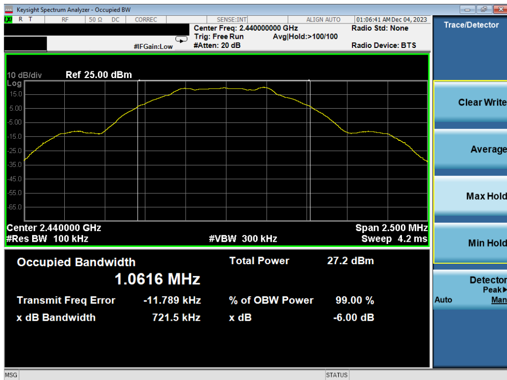
Plot 7-8. 6dB BW & 99% OBW Plot Antenna WF2b (Bluetooth (LE), 1Mbps, ePA – Ch. 19)
