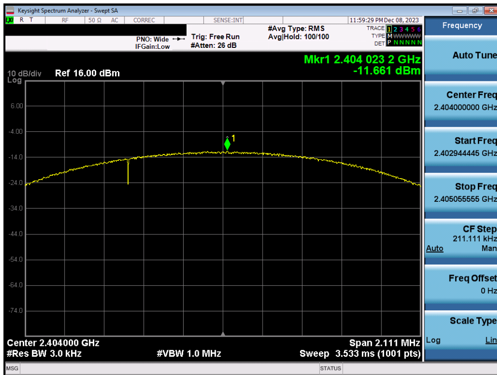
Plot 7-34. Power Spectral Density Plot Antenna WF2b (Bluetooth (LE), 2Mbps, iPA – Ch. 1)
