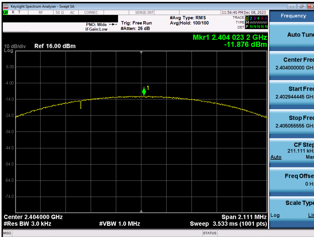
Plot 7-56. Power Spectral Density Plot Antenna WF2b (Bluetooth (LE), 2Mbps, iPA – Ch. 1)
