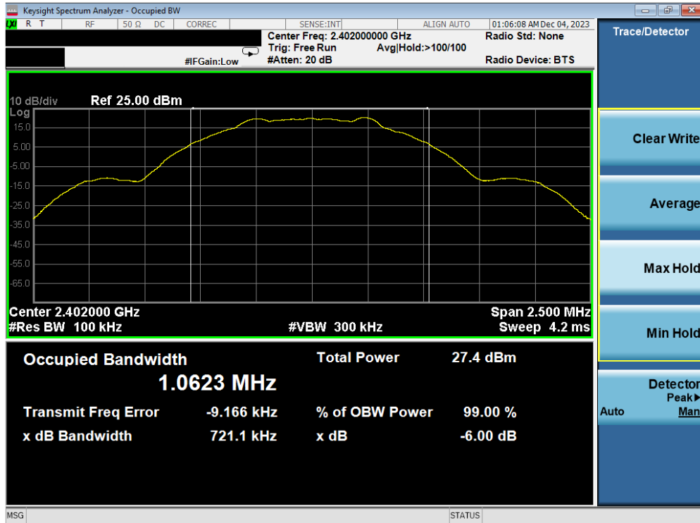
Plot 7-7. 6dB BW & 99% OBW Plot Antenna WF2b (Bluetooth (LE), 1Mbps, ePA – Ch. 0)
