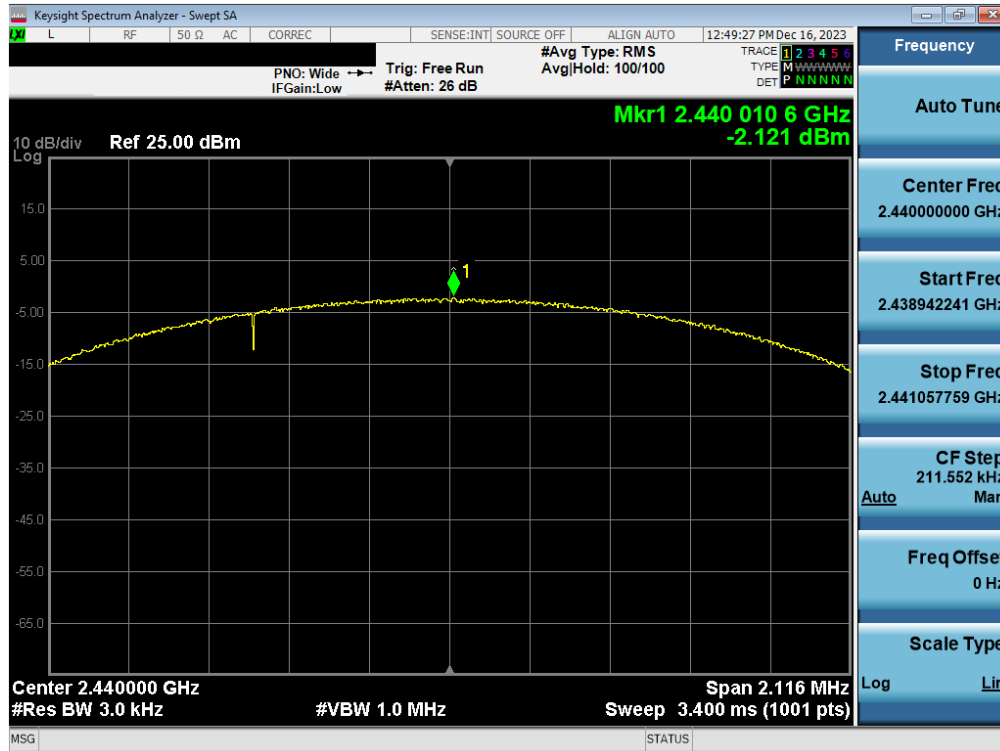
Plot 7-51. Power Spectral Density Plot Antenna WF7b (Bluetooth (LE), 2Mbps, ePA – Ch. 19)
