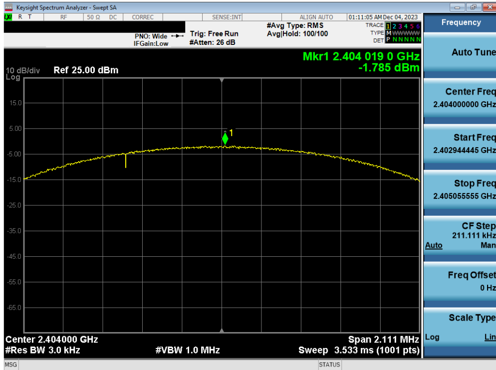
Plot 7-31. Power Spectral Density Plot Antenna WF2b (Bluetooth (LE), 2Mbps, ePA – Ch. 1)
