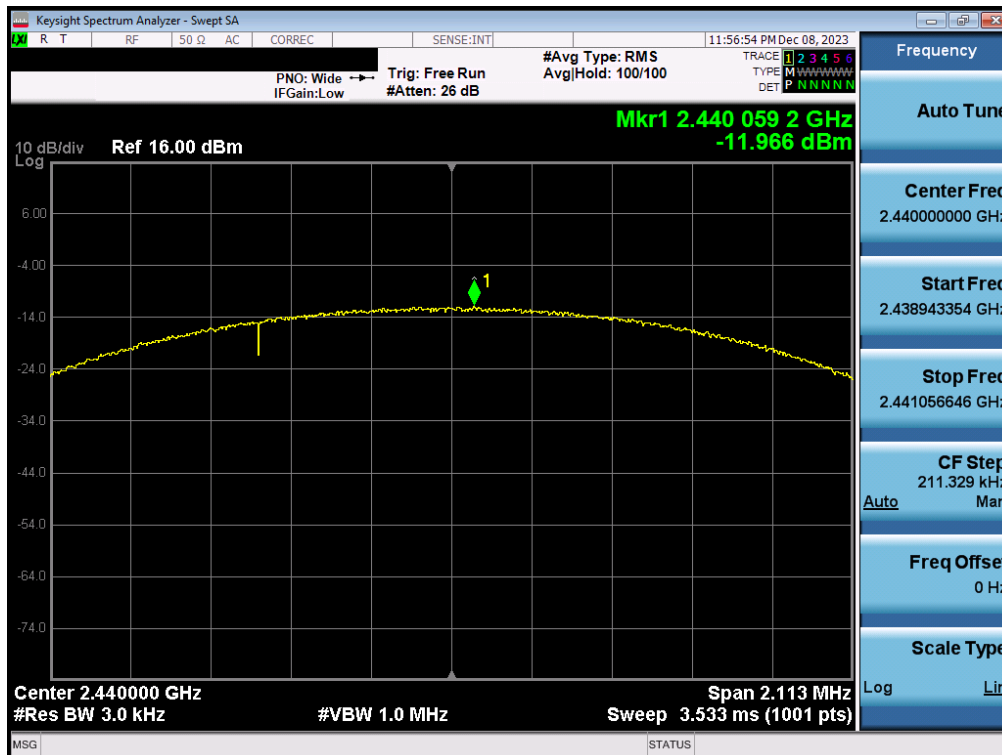
Plot 7-58. Power Spectral Density Plot Antenna WF2b (Bluetooth (LE), 2Mbps, iPA – Ch. 19)
