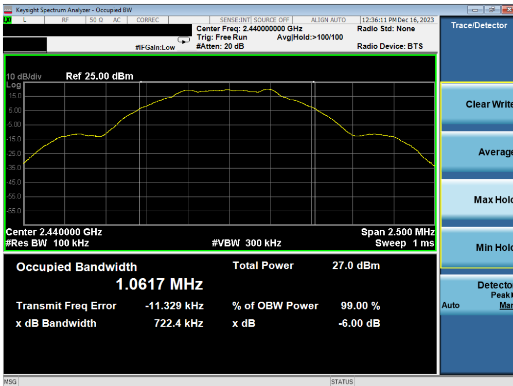
Plot 7-2. 6dB BW & 99% OBW Plot Antenna WF7b (Bluetooth (LE), 1Mbps, ePA – Ch. 19)
