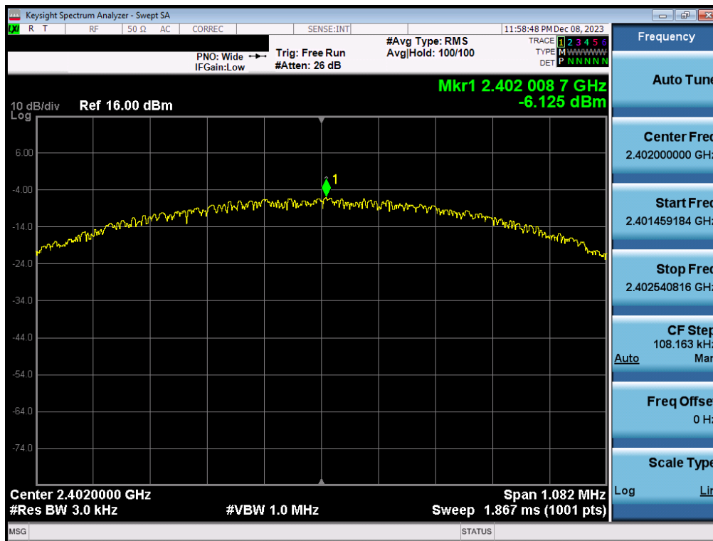
Plot 7-28. Power Spectral Density Plot Antenna WF2b (Bluetooth (LE), 1Mbps, iPA – Ch. 0)
