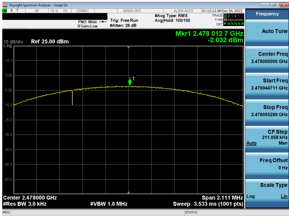
Plot 7-33. Power Spectral Density Plot Antenna WF2b (Bluetooth (LE), 2Mbps, ePA – Ch. 38)
