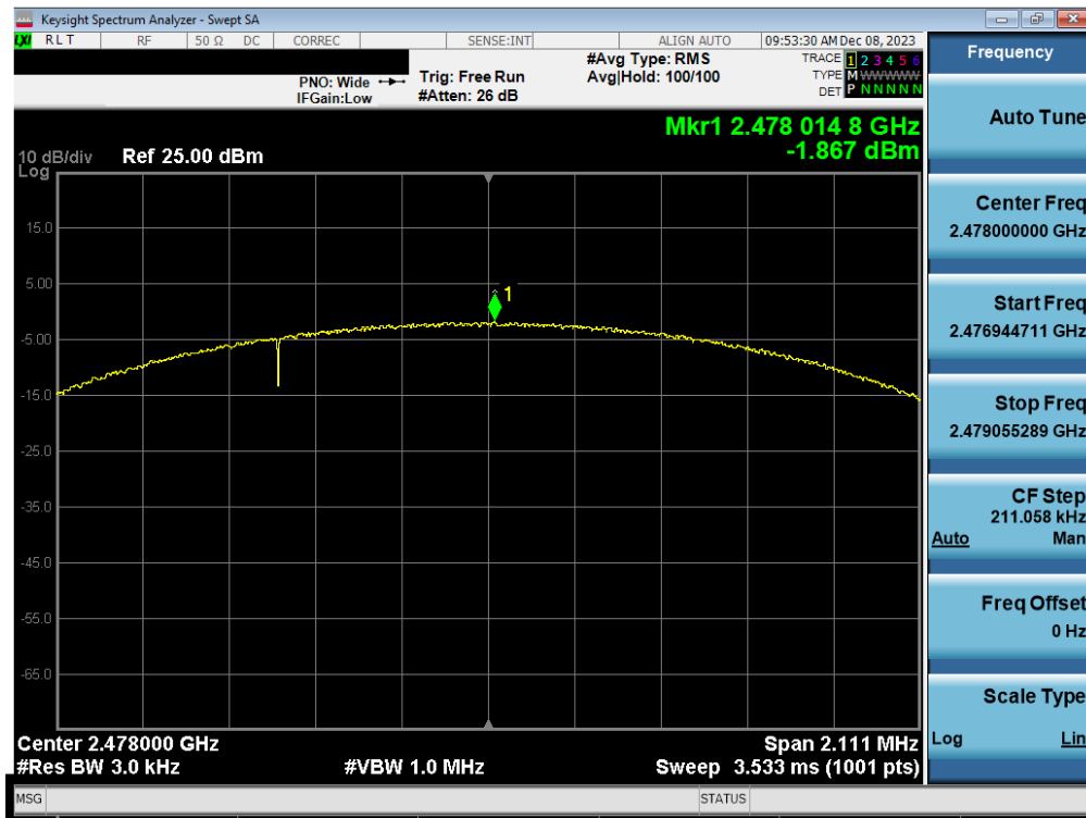
Plot 7-54. Power Spectral Density Plot Antenna WF2b (Bluetooth (LE), 2Mbps, ePA – Ch. 38)
