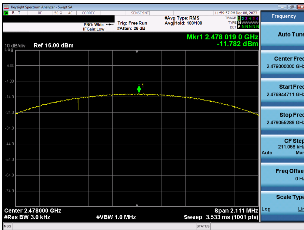
Plot 7-36. Power Spectral Density Plot Antenna WF2b (Bluetooth (LE), 2Mbps, iPA – Ch. 38)
