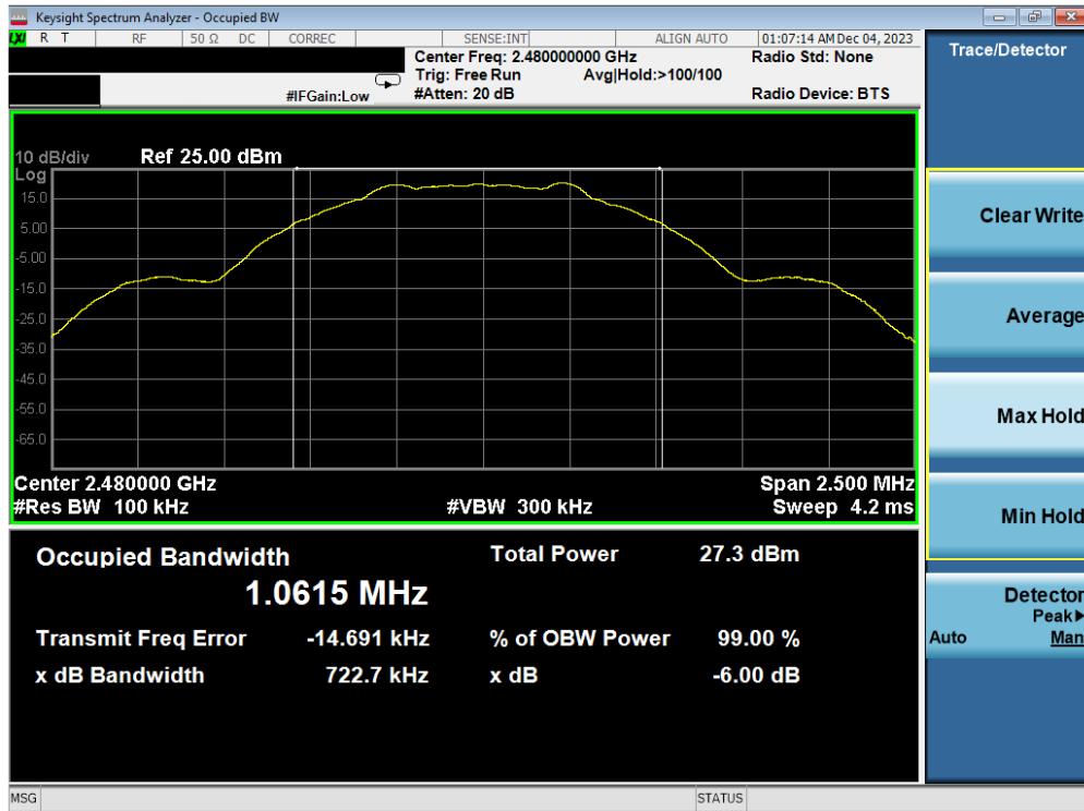
Plot 7-9. 6dB BW & 99% OBW Plot Antenna WF2b (Bluetooth (LE), 1Mbps, ePA – Ch. 39)
