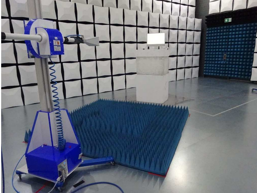
Figure 1 - Radiated Disturbance - Below 1 GHz
