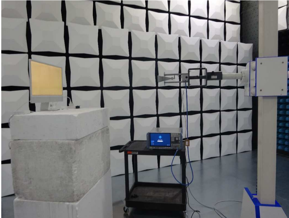
Figure 2 Radiated Disturbance - Above 1 GHz
