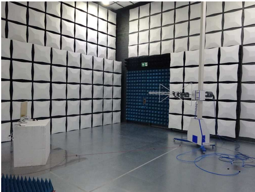
Figure 1 - Radiated Disturbance - Below 1 GHz
