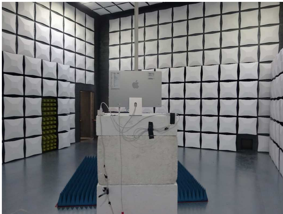
Figure 3 Radiated Disturbance - Above 1 GHz
