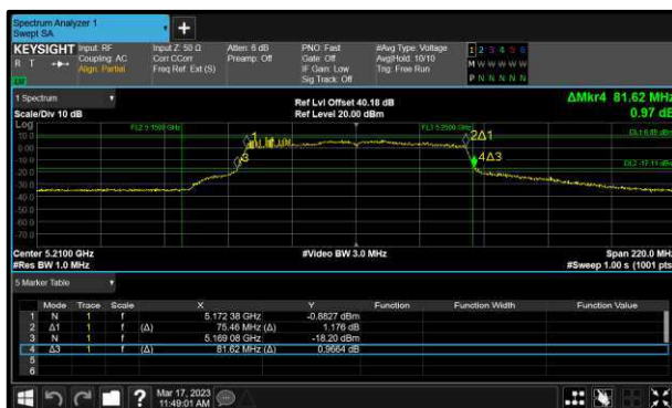
Figure 275 - 802.11ac VHT80 Minimum 99% OBW
