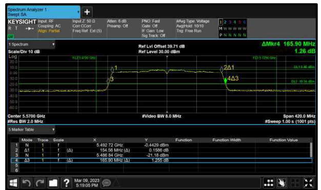
Figure 228 - 802.11ac VHT160 Maximum 99% OBW
