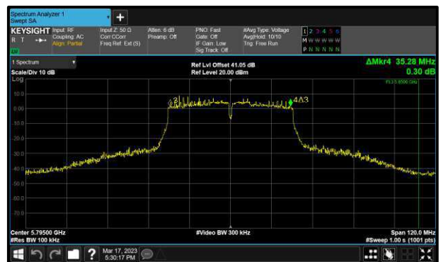
Figure 268 - 802.11ac VHT40 Maximum 6 dB EBW
