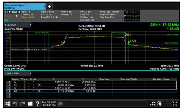
Figure 254 - 802.11ac VHT80 Maximum 99% OBW
