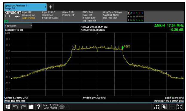
Figure 266 - 802.11ac VHT20 Maximum 6 dB EBW
