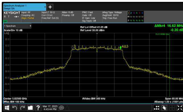
Figure 265 - 802.11ac VHT20 Minimum 6 dB EBW
