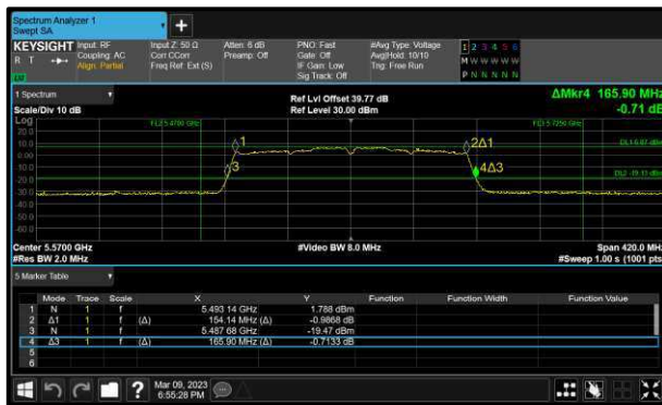
Figure 255 - 802.11ac VHT160 Minimum 99% OBW
