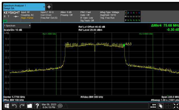
Figure 241 - 802.11ac VHT80 Minimum 6 dB EBW
