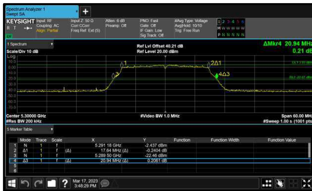
Figure 271 - 802.11ac VHT20 Minimum 99% OBW
