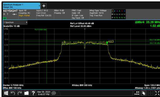
Figure 239 - 802.11n HT40 Minimum 6 dB EBW
