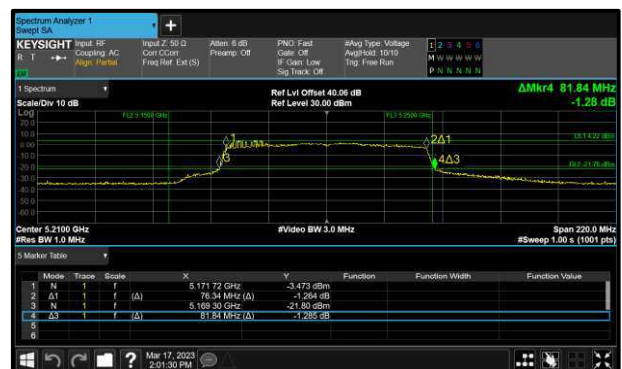
Figure 276 - 802.11ac VHT80 Maximum 99% OBW
