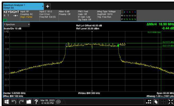
Figure 185 - 802.11ax HE20 SU Minimum 6 dB EBW
