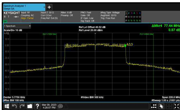
Figure 189 - 802.11ax HE80 SU Minimum 6 dB EBW
