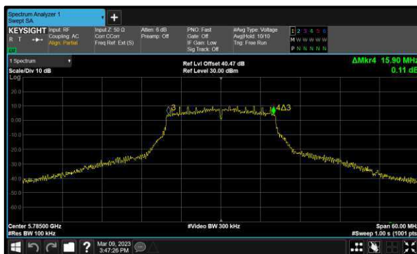
Figure 177 - 802.11a Minimum 6 dB EBW
