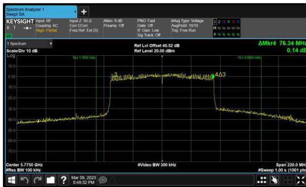
Figure 219 - 802.11ax HE80 SU Minimum 6 dB EBW
