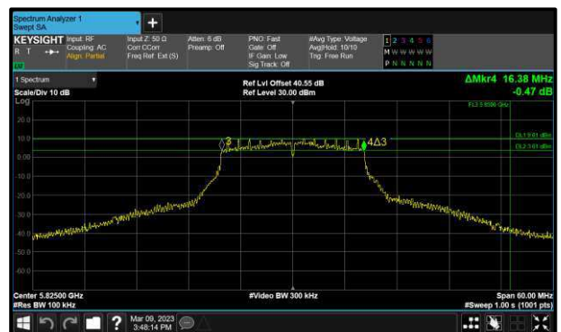
Figure 178 - 802.11a Maximum 6 dB EBW
