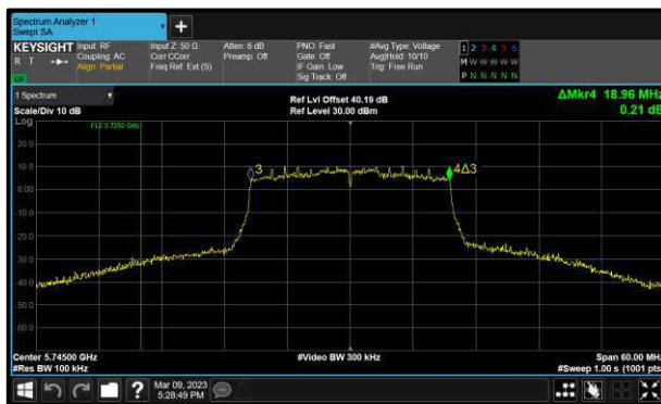
Figure 215 - 802.11ax HE20 SU Minimum 6 dB EBW
