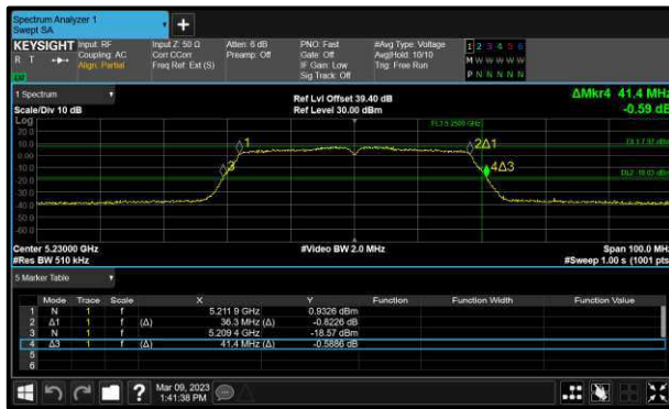
Figure 195 - 802.11n HT40 Minimum 99% OBW
