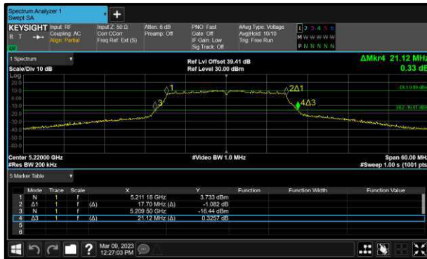
Figure 193 - 802.11n HT20 Minimum 99% OBW
