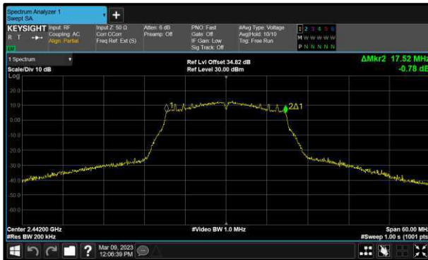
Figure 73 - 802.11n HT20 Minimum 99% OBW
