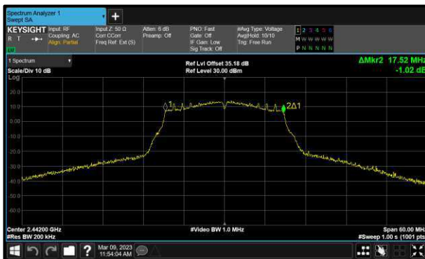
Figure 69 - 802.11n HT20 Minimum 99% OBW
