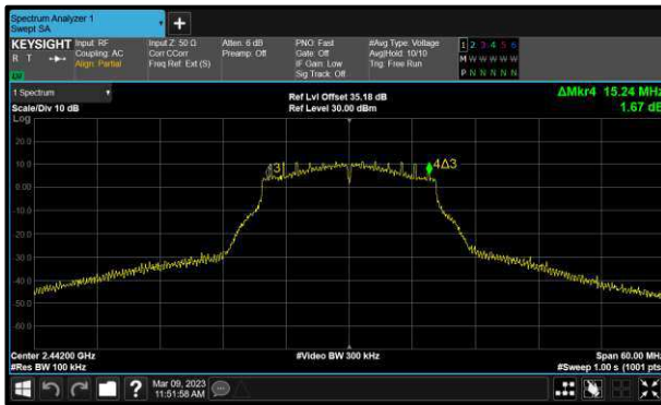
Figure 55 - 802.11g Minimum 6 dB EBW
