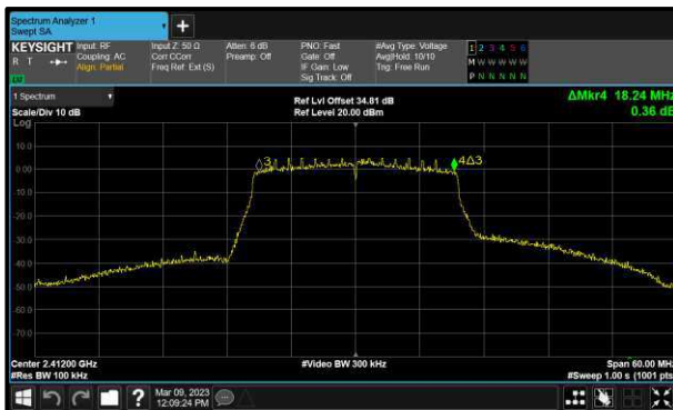
Figure 63 - 802.11ax HE20 SU Minimum 6 dB EBW
