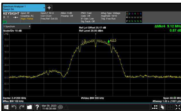
Figure 53 - 802.11b Minimum 6 dB EBW
