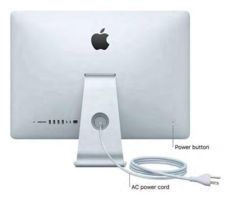
• *AC power cord*: Pass the power cord through the hole in the stand, plug it into the power port on the back of your iMac, then plug the cord into a power outlet.
