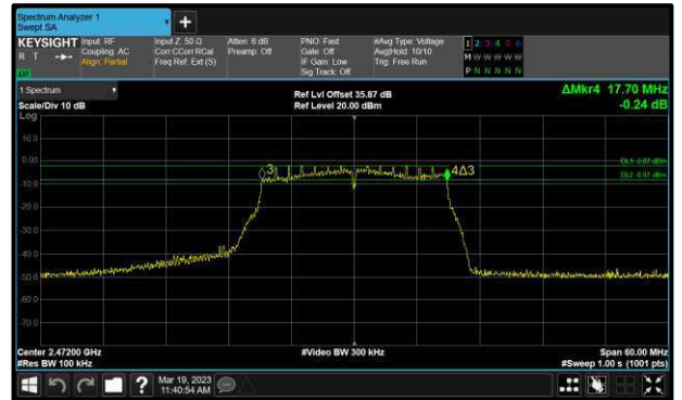
Figure 58 - 802.11n HT20 Maximum 6 dB EBW
