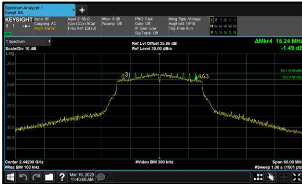
Figure 57 - 802.11n HT20 Minimum 6 dB EBW
