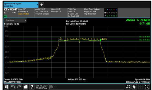
Figure 70 - 802.11n HT20 Maximum 6 dB EBW
