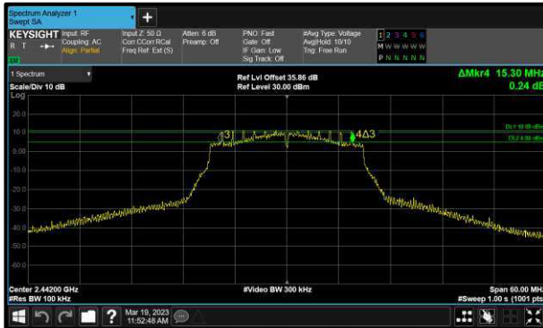
Figure 69 - 802.11n HT20 Minimum 6 dB EBW
