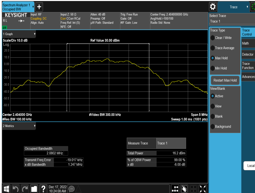
Plot 7-4. 6dB BW & 99% OBW Plot (Bluetooth (LE), 2Mbps – Ch. 1)
