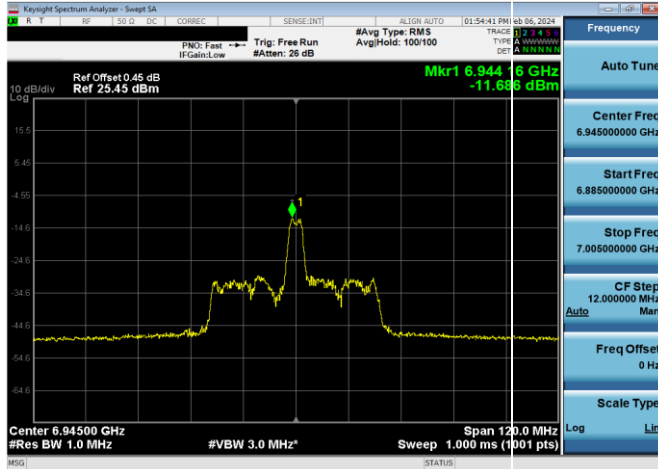
Plot 7-851. LPI Power Spectral Density Plot SDM Diversity Antenna WF5B (80MHz 802.11ax RU26 (UNII Band 8) – Ch. 199)
