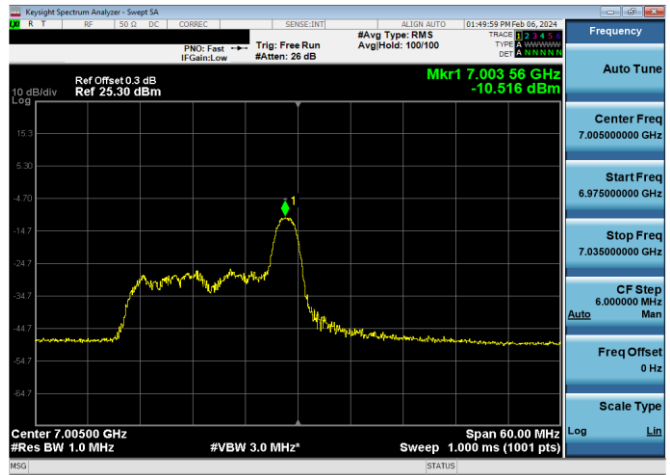
Plot 7-843. LPI Power Spectral Density Plot SDM Diversity Antenna WF5B (40MHz 802.11ax RU26 (UNII Band 8) – Ch. 211)
