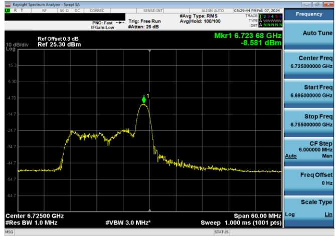
Plot 7-812. LPI Power Spectral Density Plot SDM Diversity Antenna 2a (40MHz 802.11ax RU26 (UNII Band 7) – Ch. 155)
