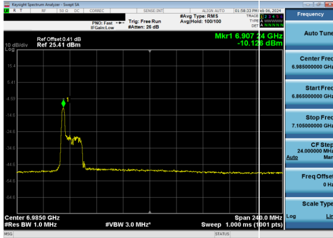
Plot 7-729. LPI Power Spectral Density Plot SDM Primary Antenna WF5B (160MHz 802.11ax RU26 (UNII Band 8) – Ch. 207)
