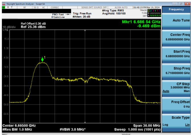
Plot 7-674. LPI Power Spectral Density Plot SDM Primary Antenna 4a (20MHz 802.11ax RU26 (UNII Band 7) – Ch. 149)
