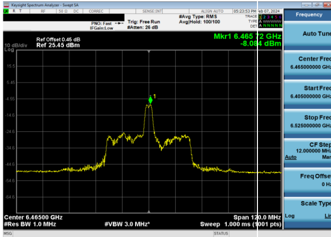
Plot 7-570. LPI Power Spectral Density Plot Antenna 2a (80MHz 802.11ax RU26 (UNII Band 6) – Ch. 103)
