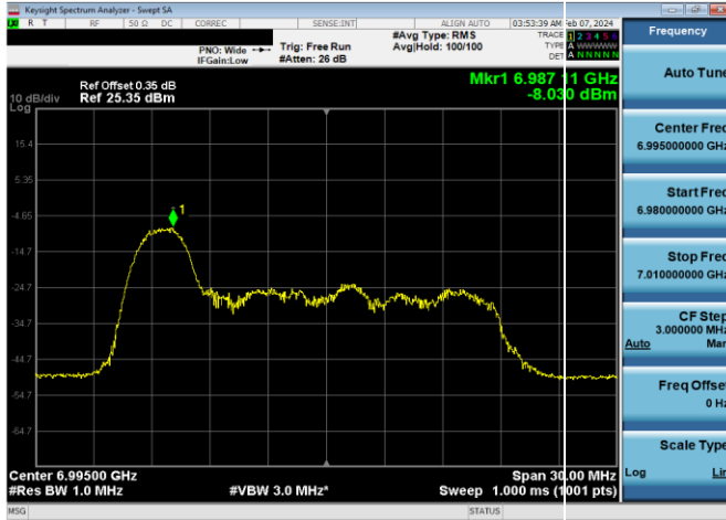
Plot 7-529. LPI Power Spectral Density Plot Antenna 4a (20MHz 802.11ax RU26 (UNII Band 8) – Ch. 209)
