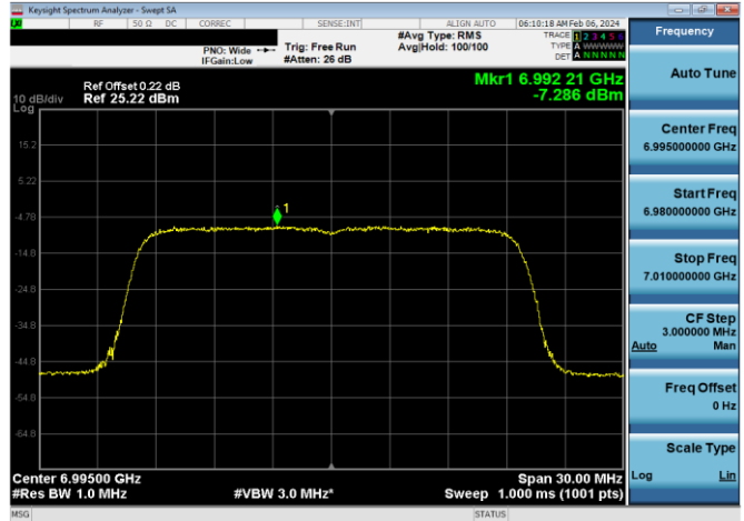
Plot 7-468. LPI Power Spectral Density Plot Antenna WF5B (20MHz 802.11ax RU242 (UNII Band 8) – Ch. 209)
