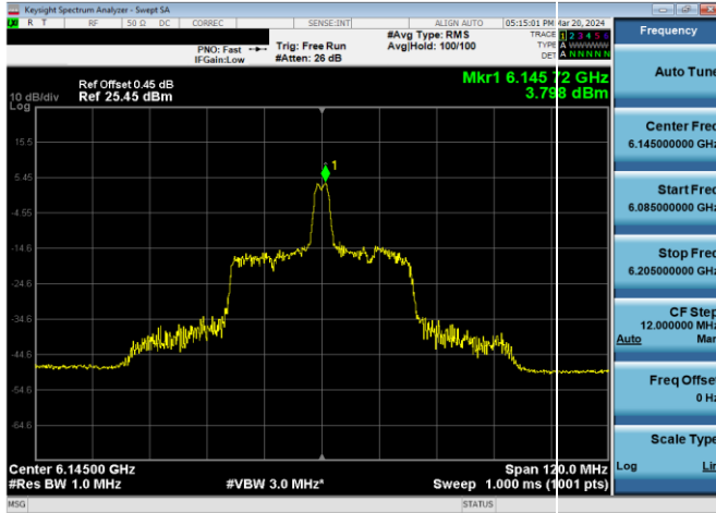
Plot 7-371. SP Power Spectral Density Plot CDD Diversity Antenna WF5B (80MHz 802.11ax RU26 (UNII Band 5) - Ch. 39)
