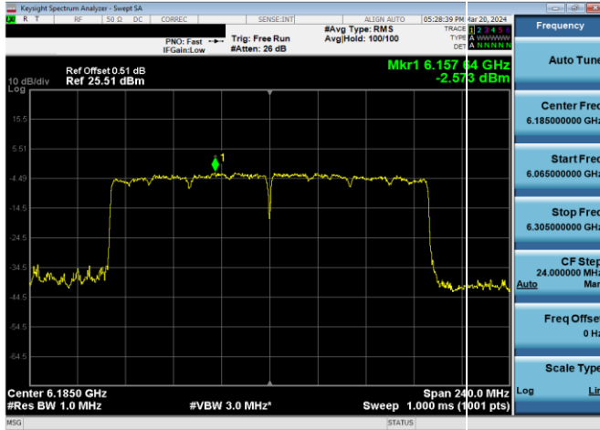
Plot 7-383. SP Power Spectral Density Plot CDD Diversity Antenna WF5B (160MHz 802.11ax RU996x2 (UNII Band 5) – Ch. 47)
