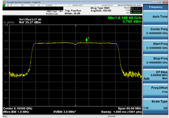
Plot 7-304. SP Power Spectral Density Plot CDD Primary Antenna 4a (40MHz 802.11ax RU484 (UNII Band 5) – Ch. 43)
