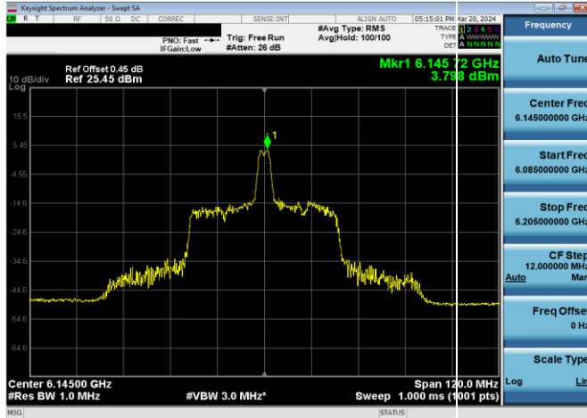
Plot 7-307. SP Power Spectral Density Plot CDD Primary Antenna WF5B (80MHz 802.11ax RU26 (UNII Band 5) - Ch. 39)
