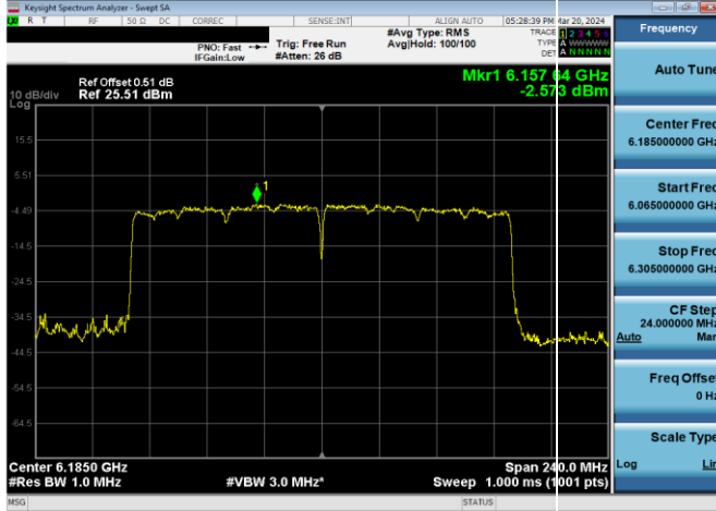
Plot 7-319. SP Power Spectral Density Plot CDD Primary Antenna WF5B (160MHz 802.11ax RU996x2 (UNII Band 5) – Ch. 47)
