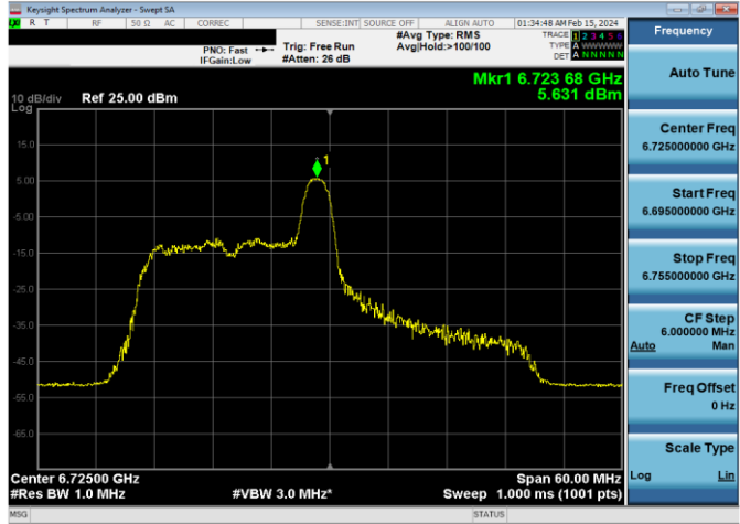
Plot 7-278. SP Power Spectral Density Plot Antenna 2a (40MHz 802.11ax RU26 (UNII Band 7) – Ch. 155)
