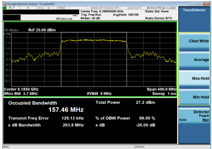
Plot 7-144. 26dB & 99% Bandwidth Plot Antenna 2a (160MHz 802.11ax RU996x2 (UNII Band 5) – Ch. 47)
