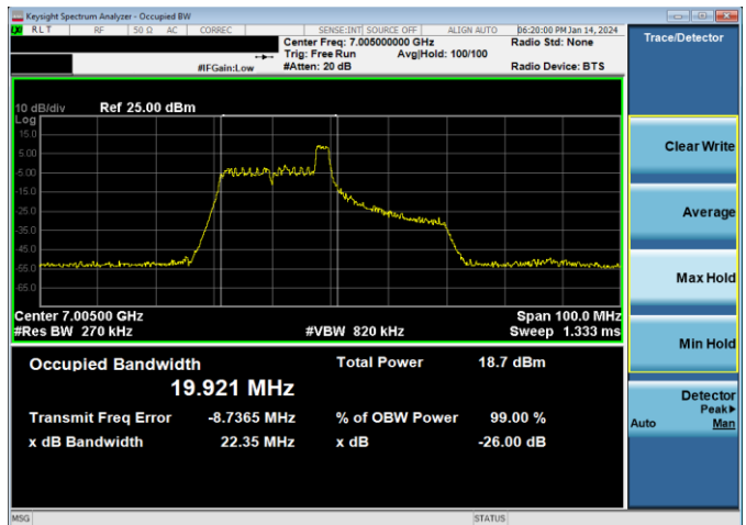
Plot 7-182. 26dB & 99% Bandwidth Plot Antenna 2a (40MHz 802.11ax RU26 (UNII Band 8) – Ch. 211)
