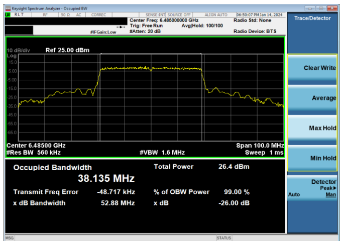
Plot 7-152. 26dB & 99% Bandwidth Plot Antenna 2a (40MHz 802.11ax RU484 (UNII Band 6) – Ch. 107)
