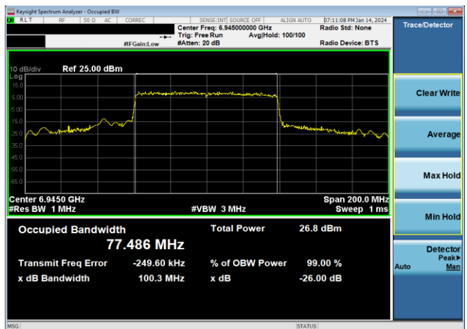
Plot 7-188. 26dB & 99% Bandwidth Plot Antenna 2a (80MHz 802.11ax RU996 (UNII Band 8) – Ch. 199)
