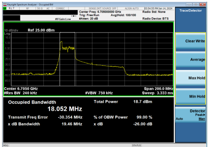
Plot 7-169. 26dB & 99% Bandwidth Plot Antenna 2a (80MHz 802.11ax RU26 (UNII Band 7) – Ch. 151)
