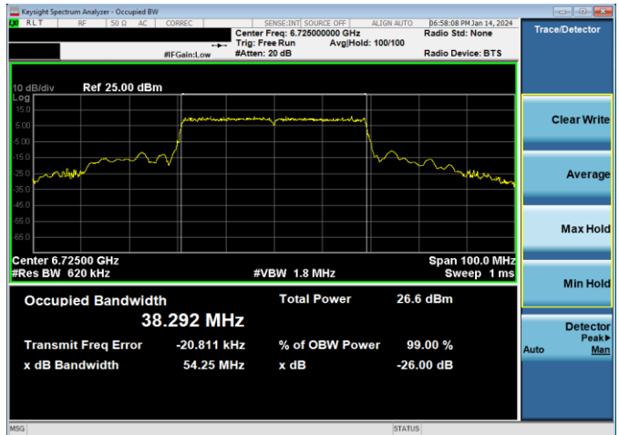
Plot 7-168. 26dB & 99% Bandwidth Plot Antenna 2a (40MHz 802.11ax RU484 (UNII Band 7) – Ch. 155)
