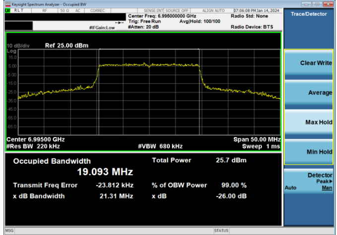
Plot 7-180. 26dB & 99% Bandwidth Plot Antenna 2a (20MHz 802.11ax RU242 (UNII Band 8) – Ch. 209)
