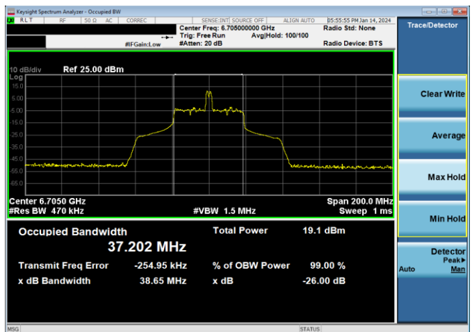
Plot 7-170. 26dB & 99% Bandwidth Plot Antenna 2a (80MHz 802.11ax RU26 (UNII Band 7) – Ch. 151)
