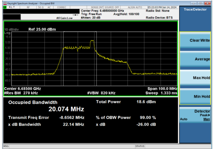
Plot 7-150. 26dB & 99% Bandwidth Plot Antenna 2a (40MHz 802.11ax RU26 (UNII Band 6) – Ch. 107)
