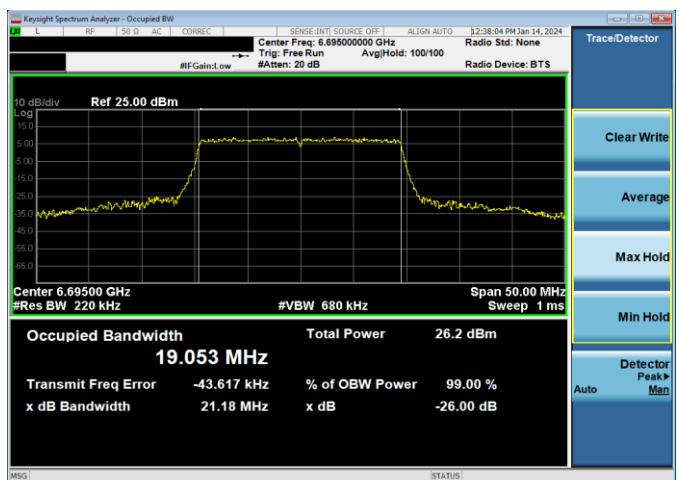
Plot 7-100. 26dB & 99% Bandwidth Plot Antenna 4a (20MHz 802.11ax RU242 (UNII Band 7) – Ch. 149)
