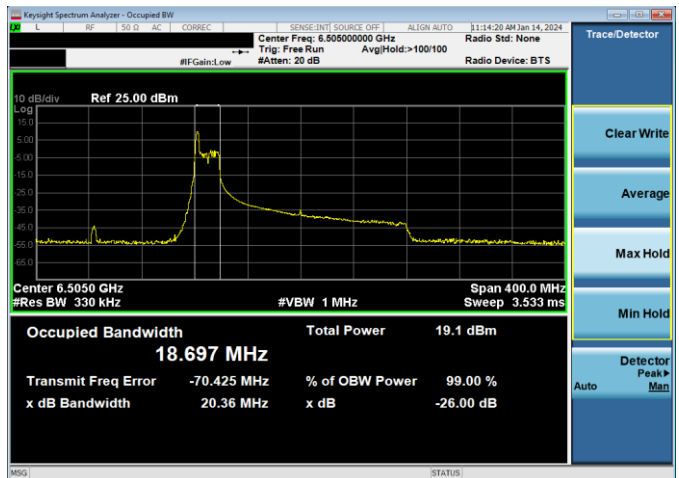
Plot 7-93. 26dB & 99% Bandwidth Plot Antenna 4a (160MHz 802.11ax RU26 (UNII Band 6) – Ch. 111)
