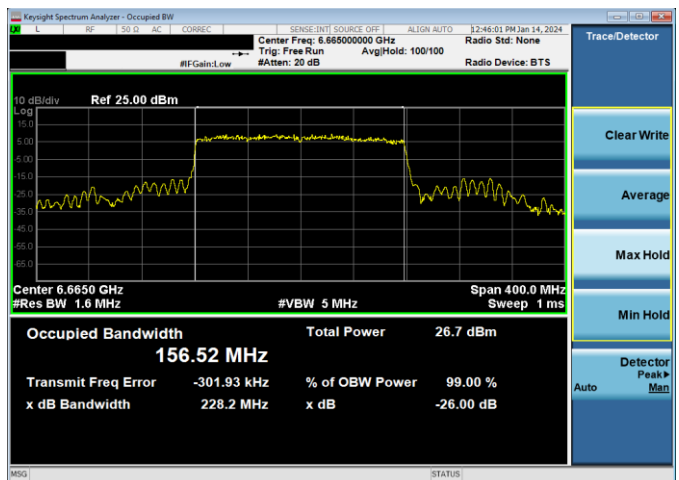
Plot 7-112. 26dB & 99% Bandwidth Plot Antenna 4a (160MHz 802.11ax RU484 (UNII Band 7) – Ch. 143)
