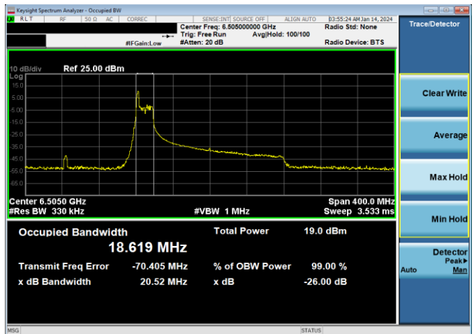
Plot 7-29. 26dB & 99% Bandwidth Plot Antenna WF5B (160MHz 802.11ax RU26 (UNII Band 6) – Ch. 111)
