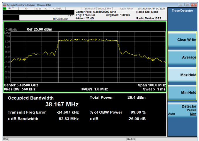
Plot 7-24. 26dB & 99% Bandwidth Plot Antenna WF5B (40MHz 802.11ax RU484 (UNII Band 6) – Ch. 107)
