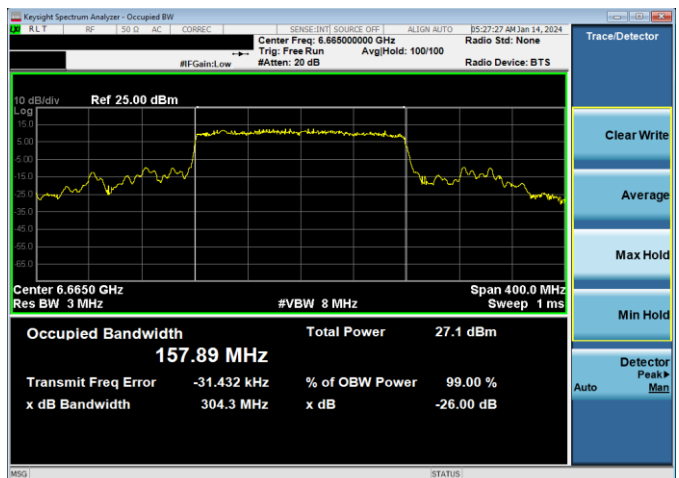
Plot 7-48. 26dB & 99% Bandwidth Plot Antenna WF5B (160MHz 802.11ax RU996x2 (UNII Band 7) – Ch. 143)
