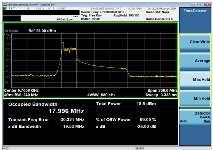
Plot 7-41. 26dB & 99% Bandwidth Plot Antenna WF5B (80MHz 802.11ax RU26 (UNII Band 7) – Ch. 151)
