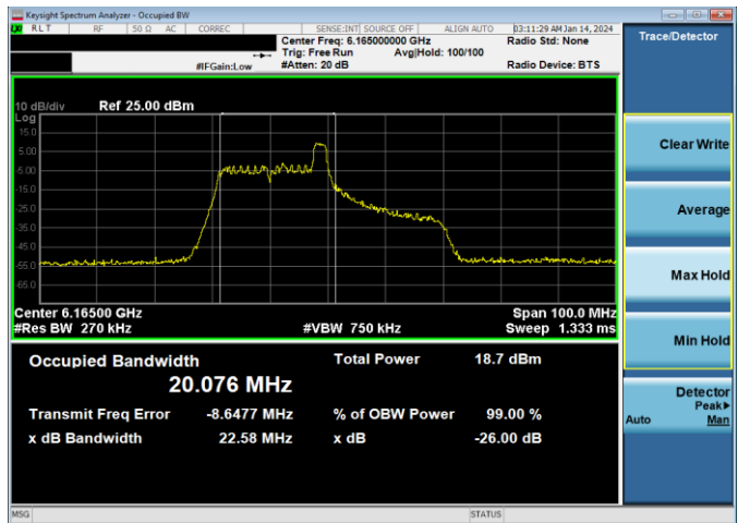
Plot 7-6. 26dB & 99% Bandwidth Plot Antenna WF5B (40MHz 802.11ax RU26 (UNII Band 5) – Ch. 43)
