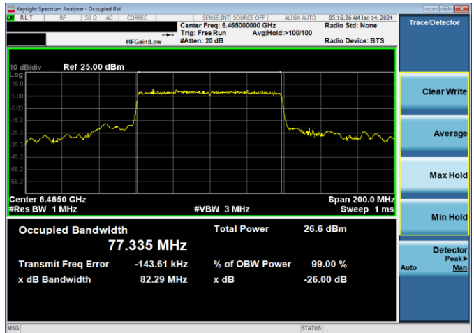
Plot 7-28. 26dB & 99% Bandwidth Plot Antenna WF5B (80MHz 802.11ax RU996 (UNII Band 6) – Ch. 103)
