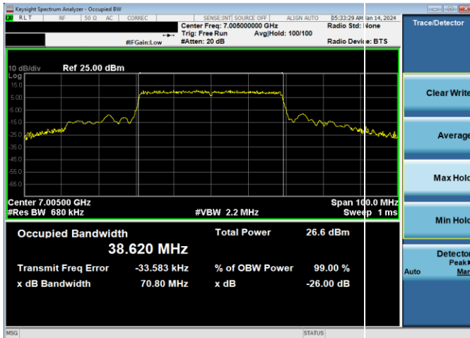
Plot 7-56. 26dB & 99% Bandwidth Plot Antenna WF5B (40MHz 802.11ax RU484 (UNII Band 8) – Ch. 211)
