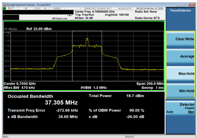
Plot 7-42. 26dB & 99% Bandwidth Plot Antenna WF5B (80MHz 802.11ax RU26 (UNII Band 7) – Ch. 151)
