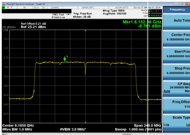
Plot 7-458. Power Spectral Density Plot SDM Primary Antenna 4a LPI (160MHz 802.11ax (UNII Band 5) – Ch. 47, MCS2)
