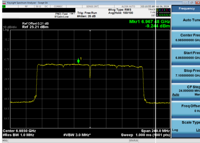
Plot 7-481. Power Spectral Density Plot SDM Primary Antenna WF5B LPI (160MHz 802.11ax (UNII Band 8) – Ch. 207, MCS2)
