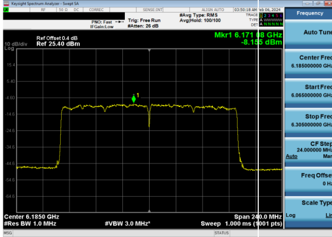
Plot 7-521. Power Spectral Density Plot SDM Primary Antenna WF5B LPI (160MHz 802.11ax (UNII Band 5) – Ch. 47, MCS11)
