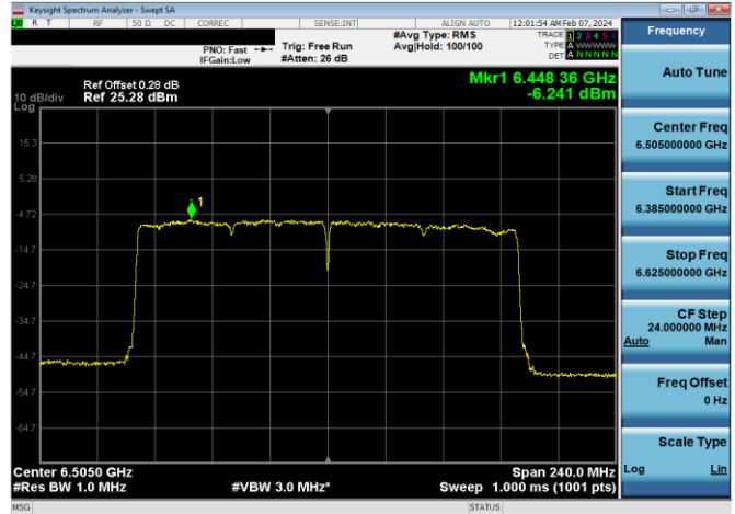
Plot 7-300. Power Spectral Density Plot Antenna 4a LPI (160MHz 802.11ax (UNII Band 6) – Ch. 111, MCS4)
