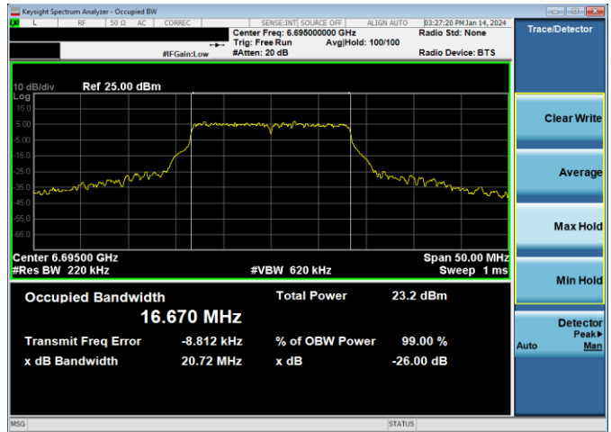
Plot 7-171. 26dB & 99% Bandwidth Plot Antenna 2a (20MHz 802.11a (UNII Band 7) – Ch. 149, 54Mbps)
