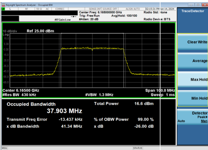
Plot 7-143. 26dB & 99% Bandwidth Plot Antenna 2a (40MHz 802.11ax (UNII Band 5) – Ch. 43, MCS4)
