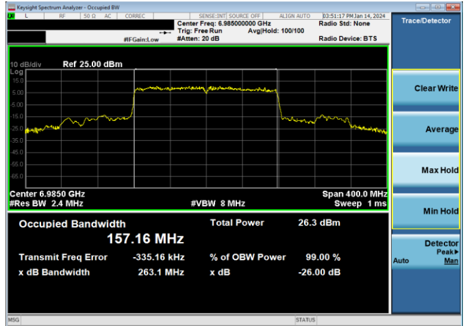
Plot 7-180. 26dB & 99% Bandwidth Plot Antenna 2a (160MHz 802.11ax (UNII Band 8) – Ch. 207, MCS11)
