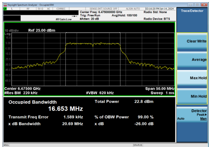
Plot 7-166. 26dB & 99% Bandwidth Plot Antenna 2a (20MHz 802.11a (UNII Band 6) – Ch. 105, 54Mbps)
