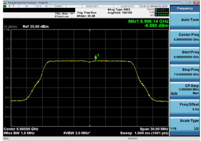
Plot 7-196. Power Spectral Density Plot Antenna WF5B LPI (20MHz 802.11a (UNII Band 8) – Ch. 209, 12Mbps)
