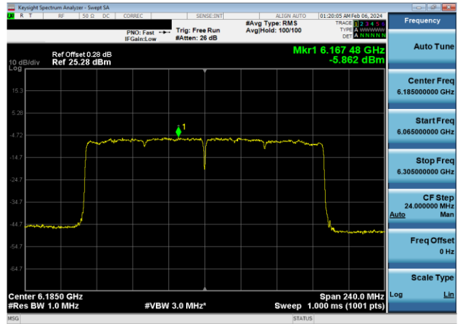
Plot 7-205. Power Spectral Density Plot Antenna WF5B LPI (160MHz 802.11ax (UNII Band 5) – Ch. 47, MCS4)
