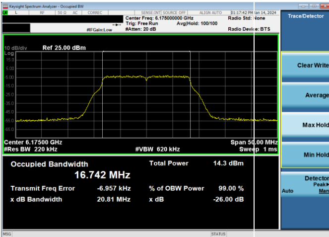
Plot 7-121. 26dB & 99% Bandwidth Plot Antenna 2a (20MHz 802.11a (UNII Band 5) – Ch. 45, 12Mbps)
