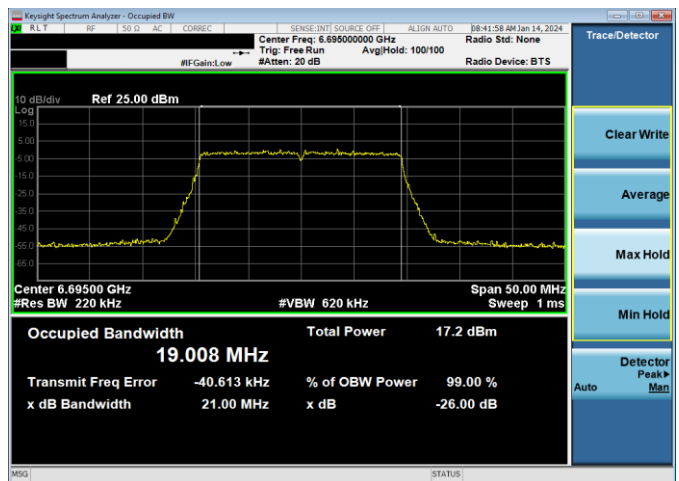
Plot 7-92. 26dB & 99% Bandwidth Plot Antenna 4a (20MHz 802.11ax (UNII Band 7) – Ch. 149, MCS4)
