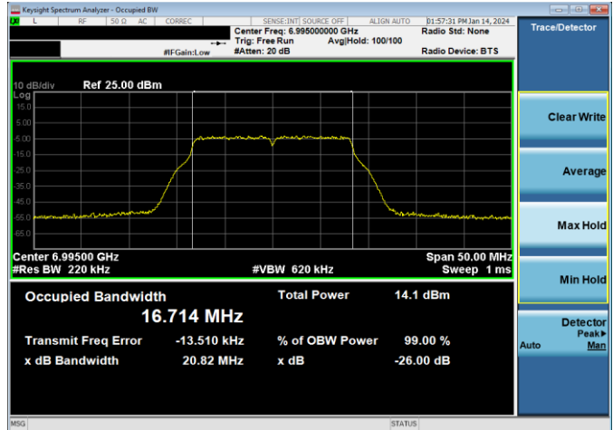
Plot 7-136. 26dB & 99% Bandwidth Plot Antenna 2a (20MHz 802.11a (UNII Band 8) – Ch. 209, 12Mbps)
