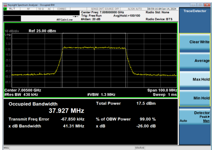
Plot 7-98. 26dB & 99% Bandwidth Plot Antenna 4a (40MHz 802.11ax (UNII Band 8) – Ch. 211, MCS4)
