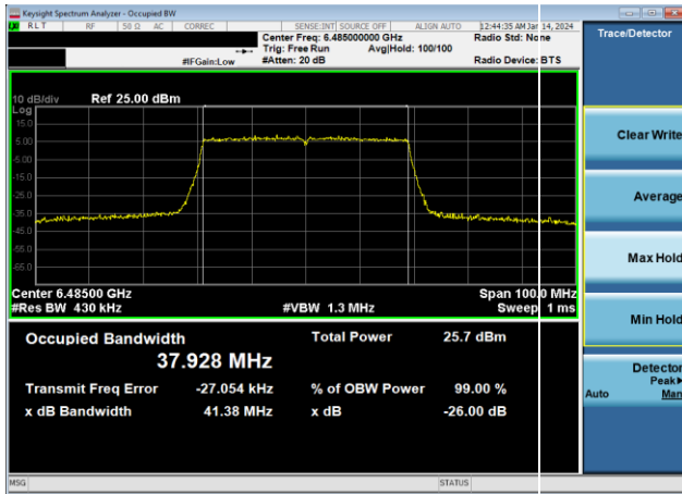
Plot 7-8. 26dB & 99% Bandwidth Plot Antenna WF5B (40MHz 802.11ax (UNII Band 6) – Ch. 107, MCS2)
