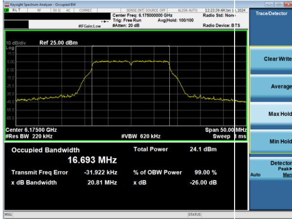
Plot 7-1. 26dB & 99% Bandwidth Plot Antenna WF5B (20MHz 802.11a (UNII Band 5) – Ch. 45, 12Mbps)
