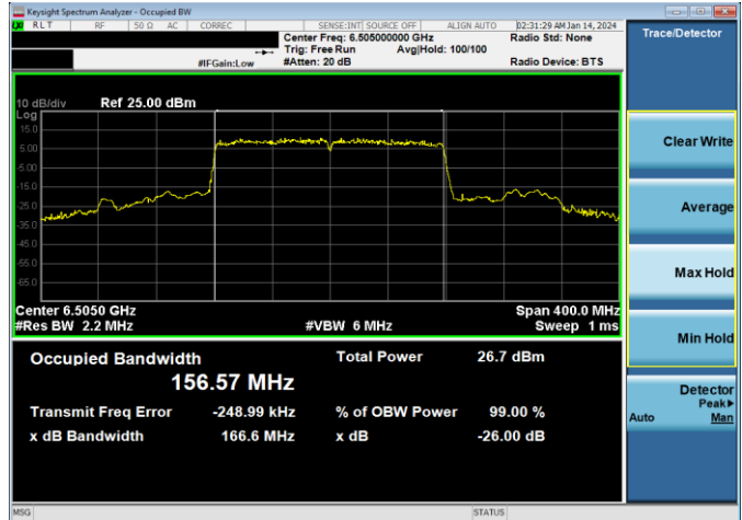
Plot 7-50. 26dB & 99% Bandwidth Plot Antenna WF5B (160MHz 802.11ax (UNII Band 6) – Ch. 111, MCS11)
