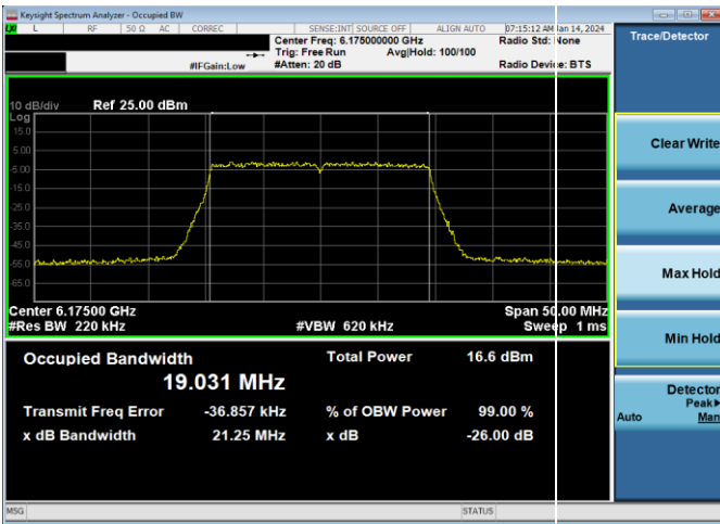
Plot 7-62. 26dB & 99% Bandwidth Plot Antenna 4a (20MHz 802.11ax (UNII Band 5) – Ch. 45, MCS2)
