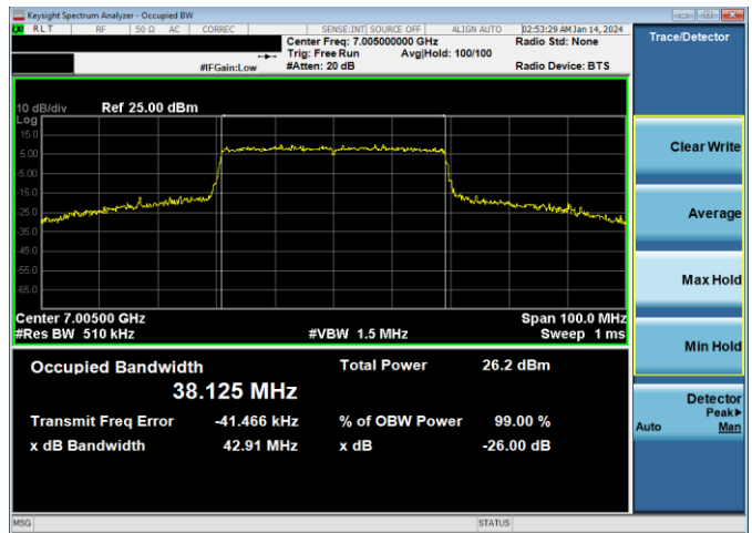
Plot 7-58. 26dB & 99% Bandwidth Plot Antenna WF5B (40MHz 802.11ax (UNII Band 8) – Ch. 211, MCS11)
