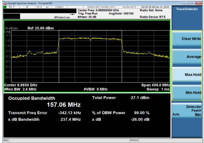
Plot 7-40. 26dB & 99% Bandwidth Plot Antenna WF5B (160MHz) 802.11ax (UNII Band 8) – Ch. 207, MCS4)
