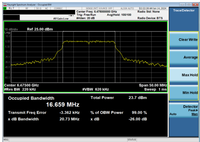
Plot 7-46. 26dB & 99% Bandwidth Plot Antenna WF5B (20MHz 802.11a (UNII Band 6) – Ch. 105, 54Mbps)
