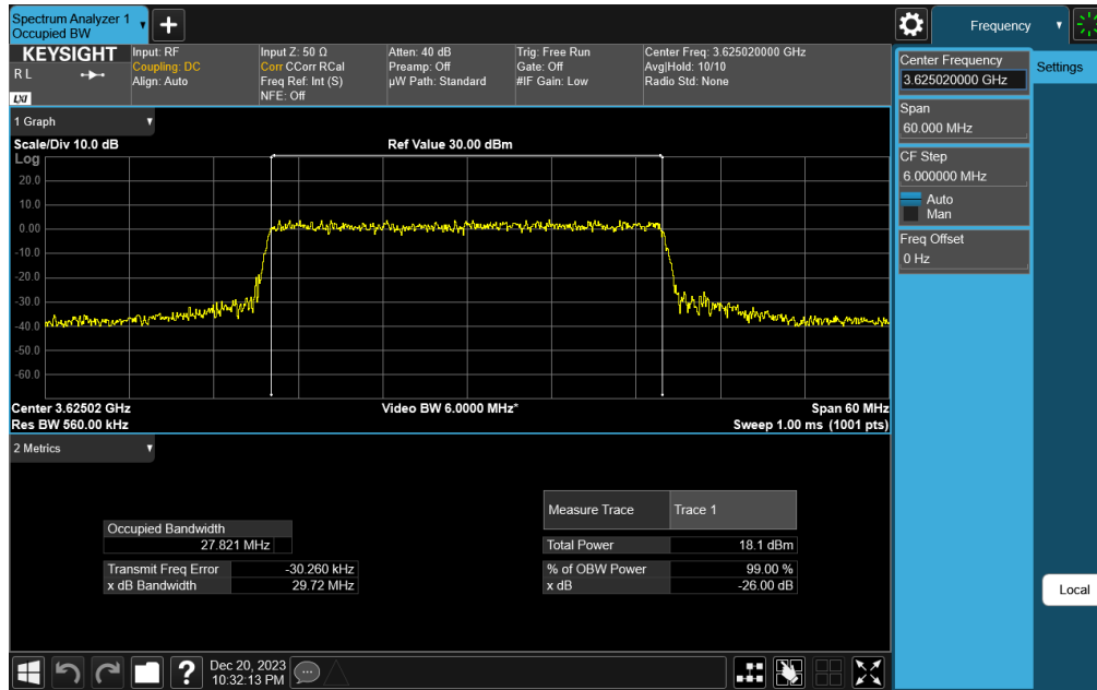
Plot 7-51. Occupied Bandwidth Plot (NR Band n48 - 30MHz 64-QAM - Full RB Configuration)
