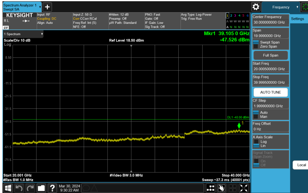
Plot 7-84. Conducted Spurious Plot (NR Band n48 - 40MHz QPSK - Low Channel)
