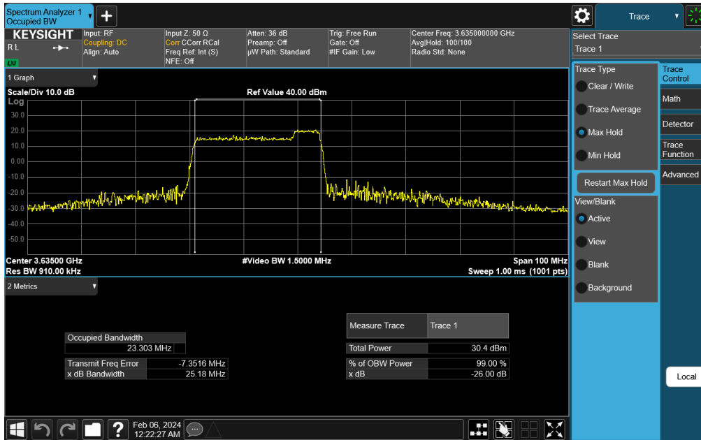
Plot 7-18. Occupied Bandwidth Plot (ULCA LTE Band 48 - 20+5MHz 16-QAM - Full RB Configuration)
