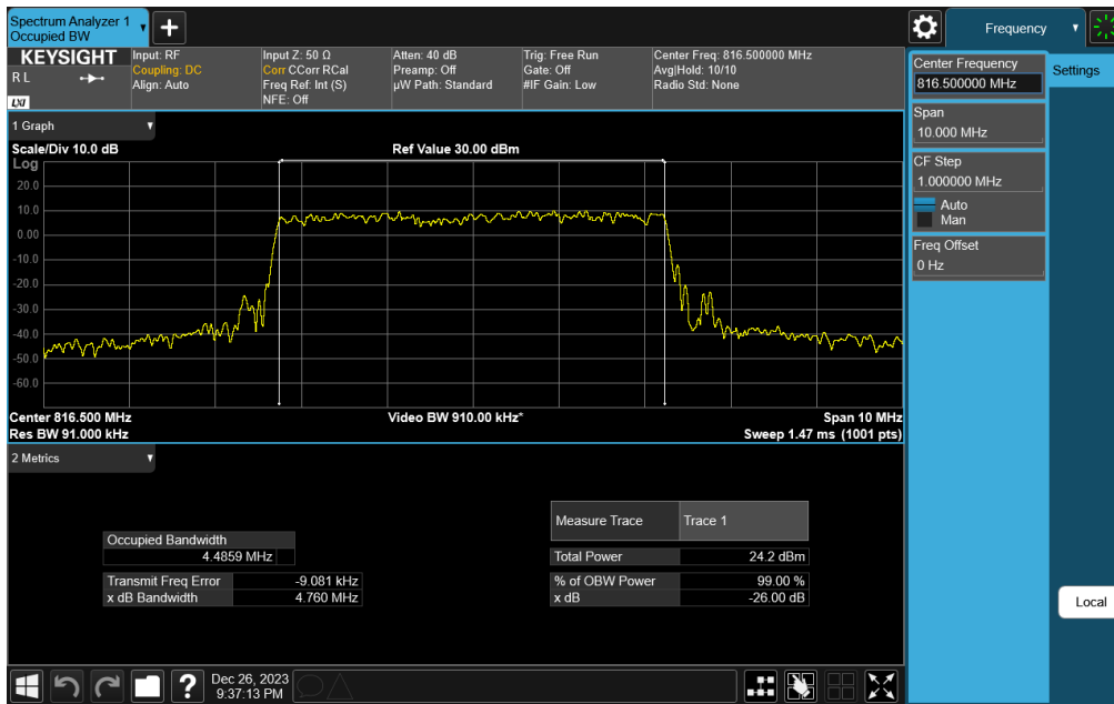
Plot 7-36. Occupied Bandwidth Plot (NR Band 26 - 5MHz DFT-s-OFDM QPSK - Full RB)
