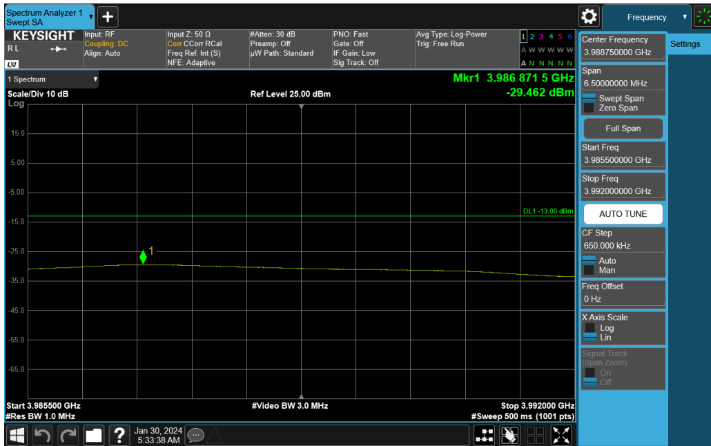
Plot 7-288. Upper ACP Plot (NR Band n77 C-Band - 80MHz DFT-s-OFDM QPSK – Full RB)
