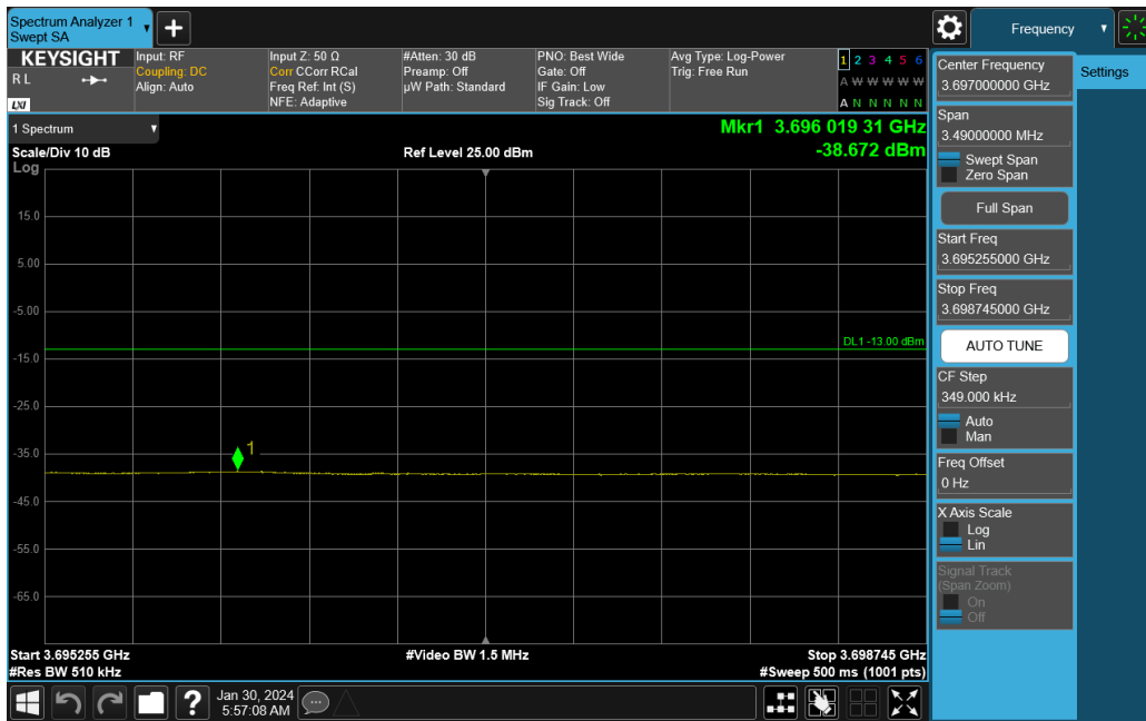
Plot 7-298. Lower ACP Plot (NR Band n77 C-Band - 100MHz DFT-s-OFDM QPSK – Full RB)
