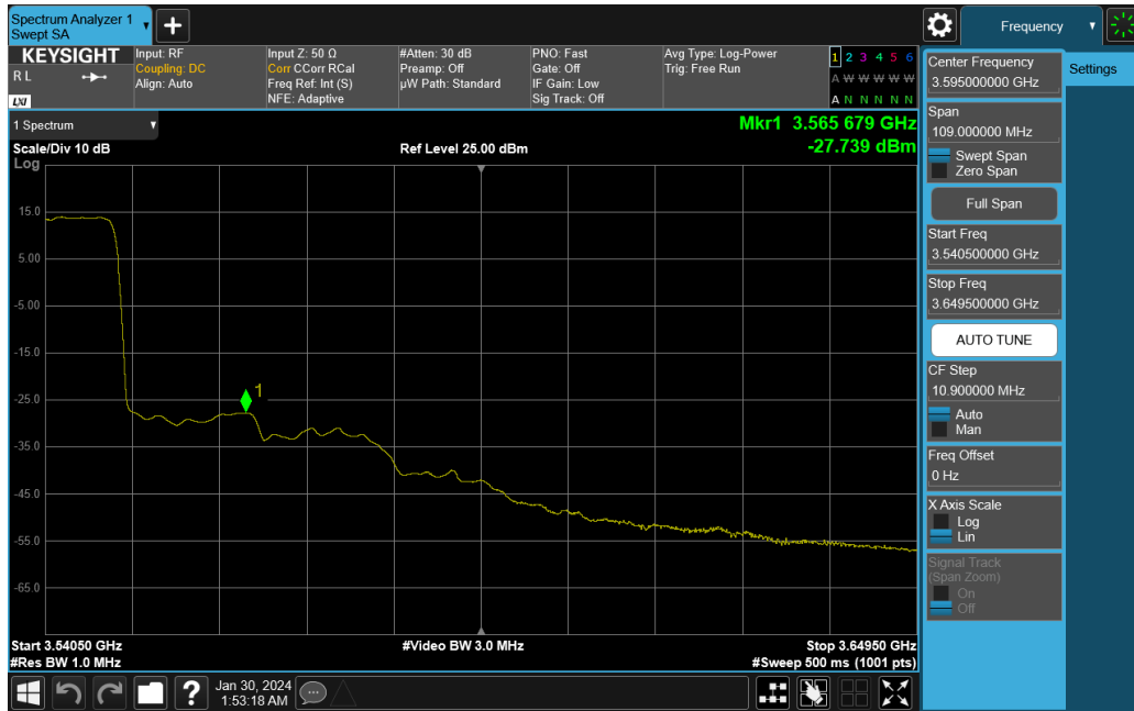
Plot 7-149. Upper ACP Plot (NR Band n77 DoD-Band - 20MHz DFT-s-OFDM QPSK – Full RB)
