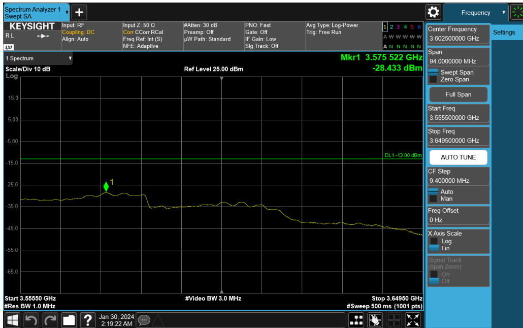
Plot 7-168. Upper ACP Plot (NR Band n77 DoD-Band - 40MHz DFT-s-OFDM QPSK – Full RB)
