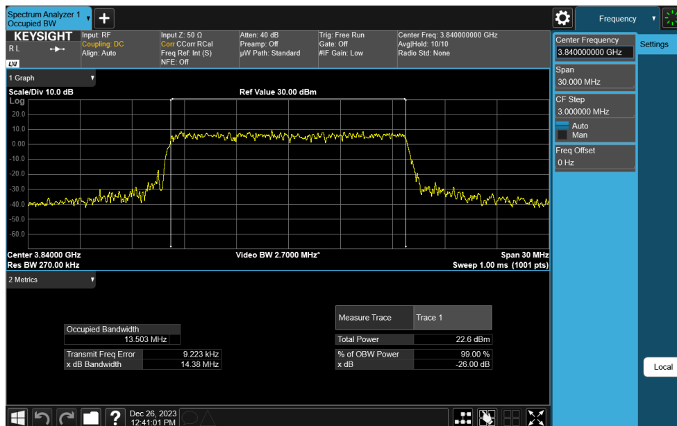
Plot 7-63. Occupied Bandwidth Plot (NR Band n77 C-Band - 15MHz CP-OFDM 16-QAM - Full RB)
