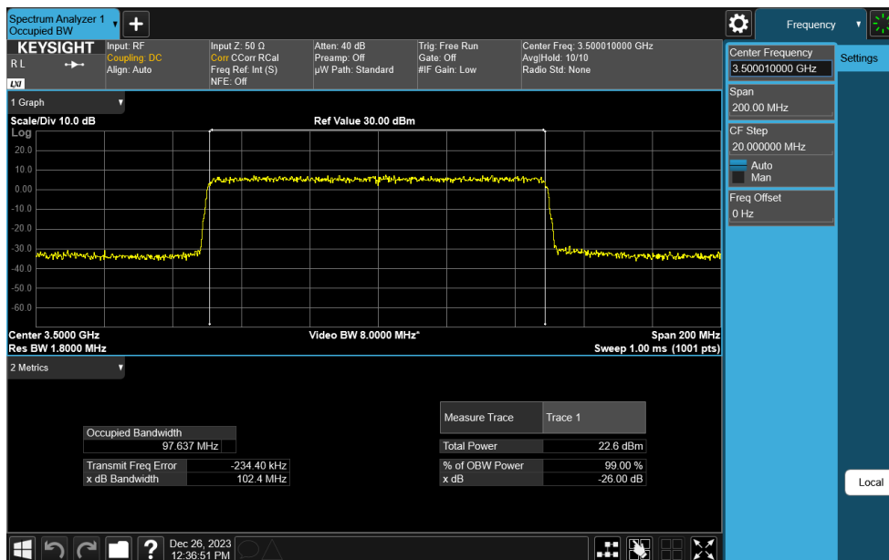
Plot 7-54. Occupied Bandwidth Plot (NR Band n77 DoD-Band - 100MHz CP-OFDM 64-QAM - Full RB)
