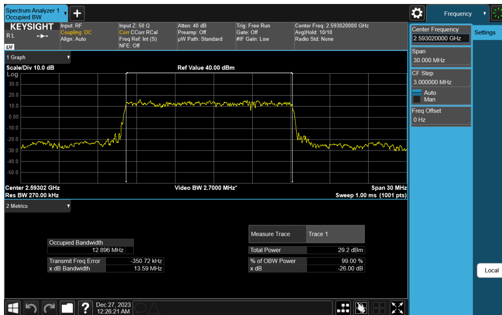
Plot 7-96. Occupied Bandwidth Plot (NR Band n41 - 15MHz DFT-s-OFDM \pi/2 BPSK - Full RB)
