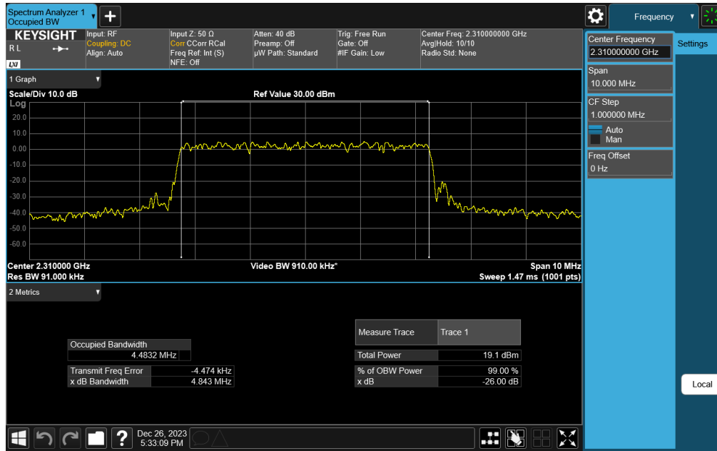
Plot 7-45. Occupied Bandwidth Plot (NR Band n30 - 5MHz CP-OFDM 256-QAM - Full RB)
