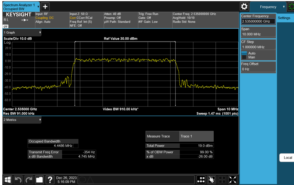
Plot 7-55. Occupied Bandwidth Plot (NR Band n7 - 5MHz CP-OFDM 256-QAM - Full RB)
