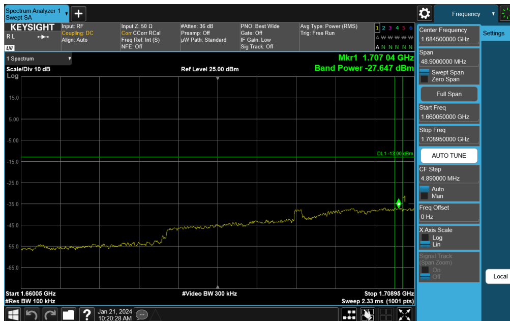
Plot 7-337. Lower Extended Band Edge Plot (NR Band n66 – 35.0MHz DFT-s-OFDM \pi/2 BPSK - Full RB)
