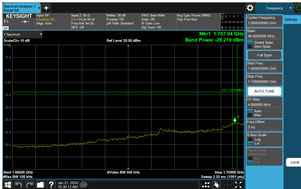
Plot 7-341. Lower Extended Band Edge Plot (NR Band n66 – 40.0MHz DFT-s-OFDM \pi/2 BPSK - Full RB)
