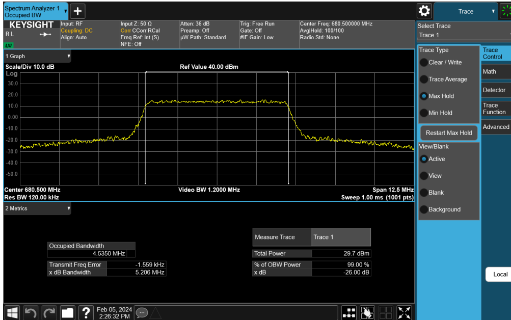
Plot 7-26. Occupied Bandwidth Plot (LTE Band 71 - 5MHz 16-QAM - Full RB)
