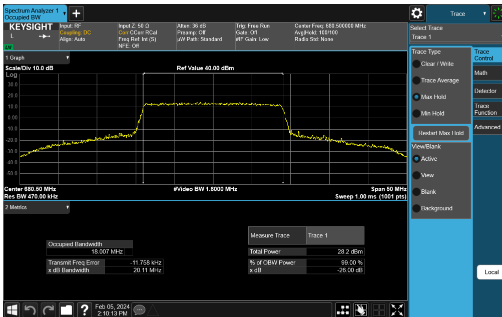
Plot 7-38. Occupied Bandwidth Plot (LTE Band 71 - 20MHz 16-QAM - Full RB)
