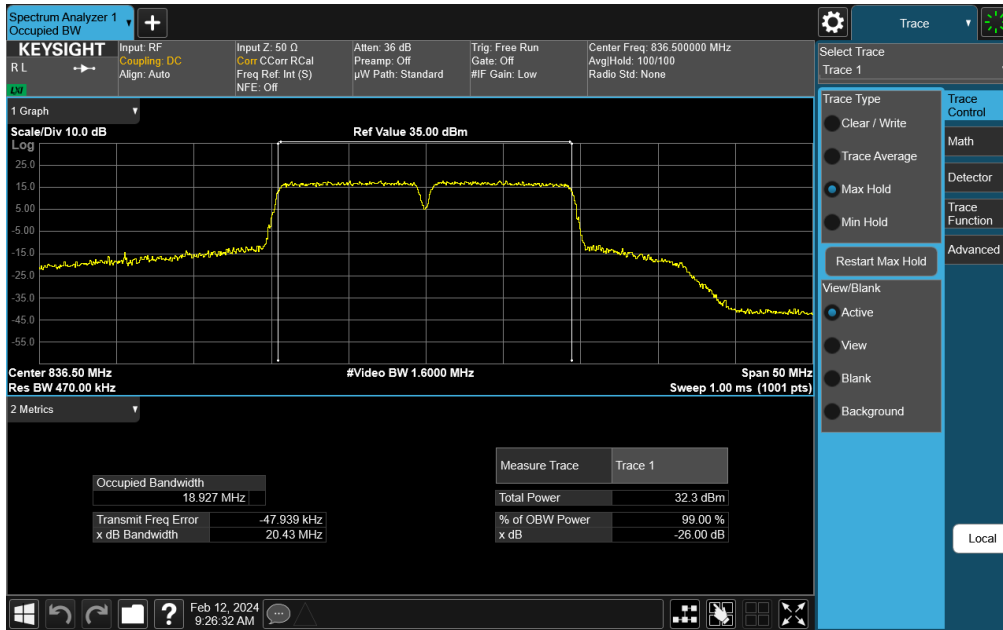
Plot 7-17. Conducted Spurious Plot (ULCA LTE Band 5 – (10 + 10)MHz QPSK - Full RB Configuration)
