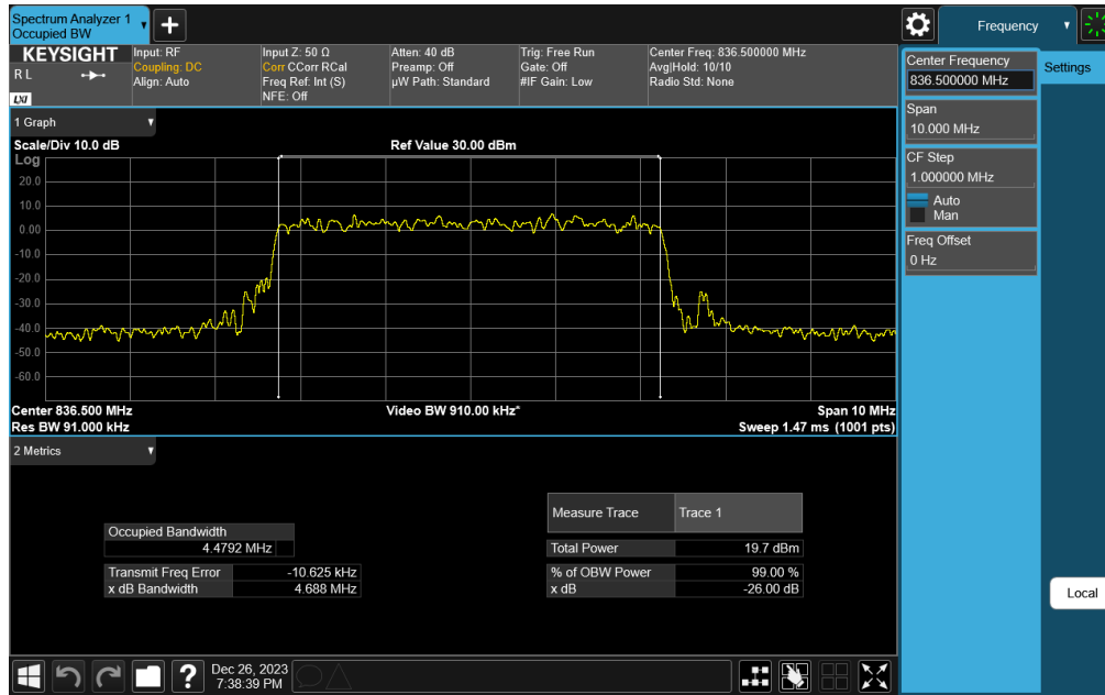
Plot 7-25. Occupied Bandwidth Plot (NR Band n26/n5 - 5MHz CP-OFDM 256-QAM - Full RB Configuration)
