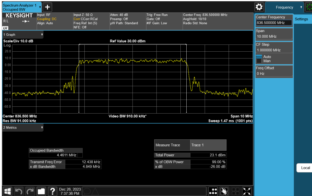
Plot 7-23. Occupied Bandwidth Plot (NR Band n26/n5 - 5MHz CP-OFDM 16-QAM - Full RB Configuration)
