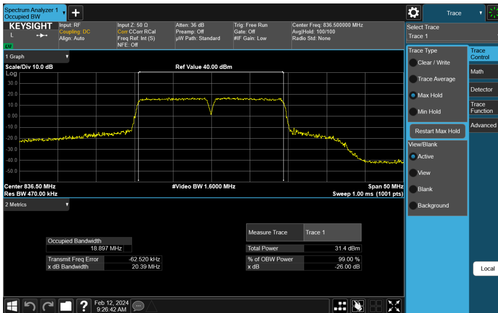
Plot 7-18. Conducted Spurious Plot (ULCA LTE Band 5 – (10 + 10)MHz 16-QAM - Full RB Configuration)
