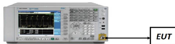
Figure 7-5. Test Instrument & Measurement Setup
