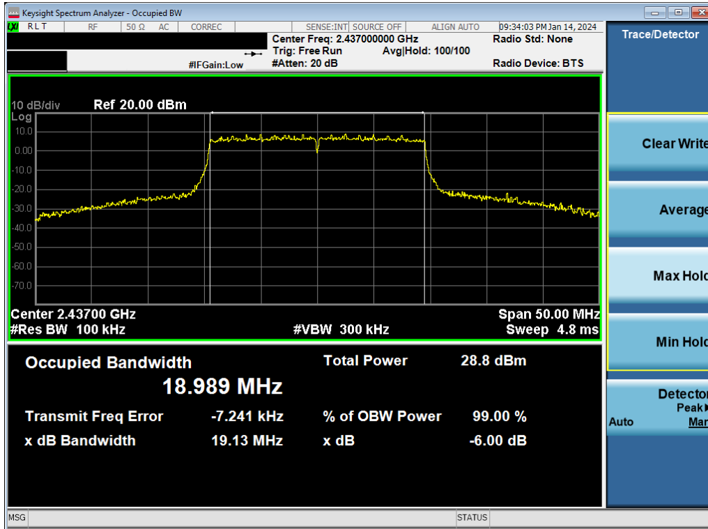
Plot 7-11. 6dB BW & 99% OBW Plot Antenna 4a (802.11ax OFDMA – RU242 – Ch. 6)
