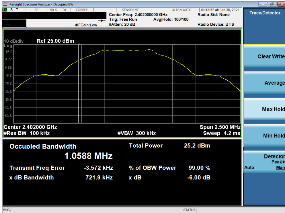
Plot 7-7. 6dB BW & 99% OBW Plot Antenna 2a (Bluetooth (LE), 1Mbps, ePA – Ch. 0)
