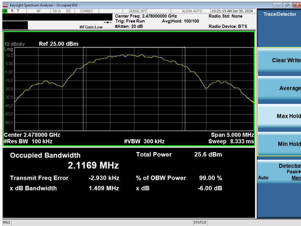
Plot 7-6. 6dB BW & 99% OBW Plot Antenna 4a (Bluetooth (LE), 2Mbps, ePA – Ch. 38)
