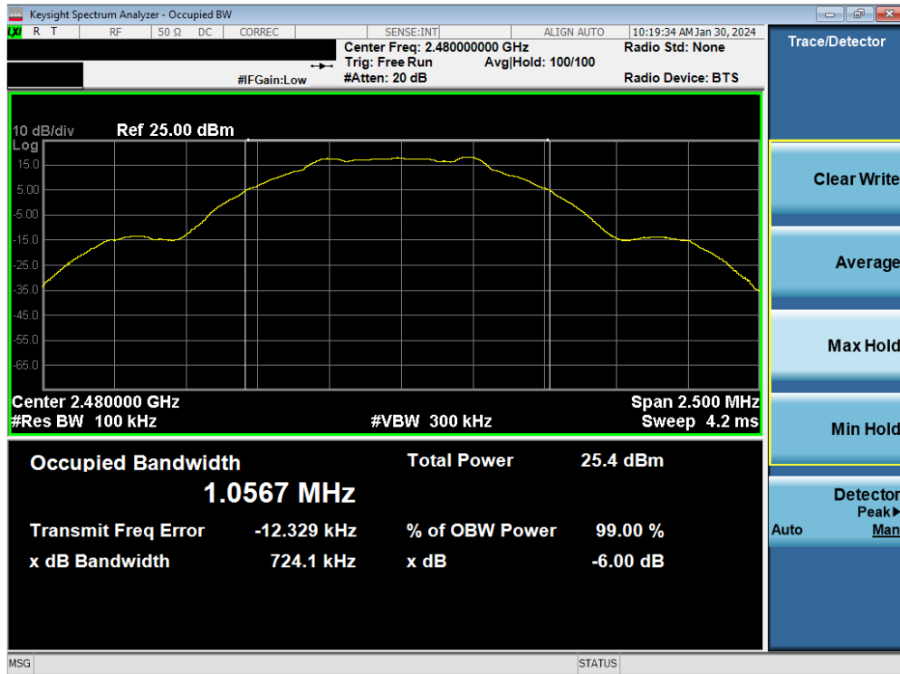
Plot 7-3. 6dB BW & 99% OBW Plot Antenna 4a (Bluetooth (LE), 1Mbps, ePA – Ch. 39)
