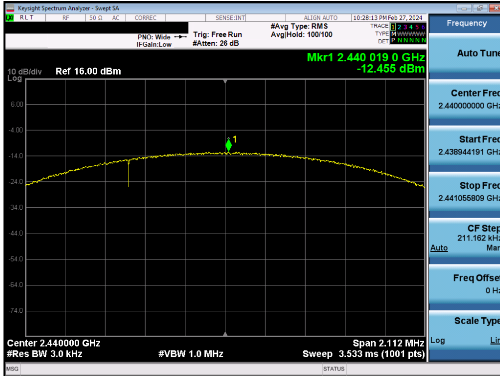
Plot 7-35. Power Spectral Density Plot Antenna 2a (Bluetooth (LE), 2Mbps, iPA – Ch. 19)
