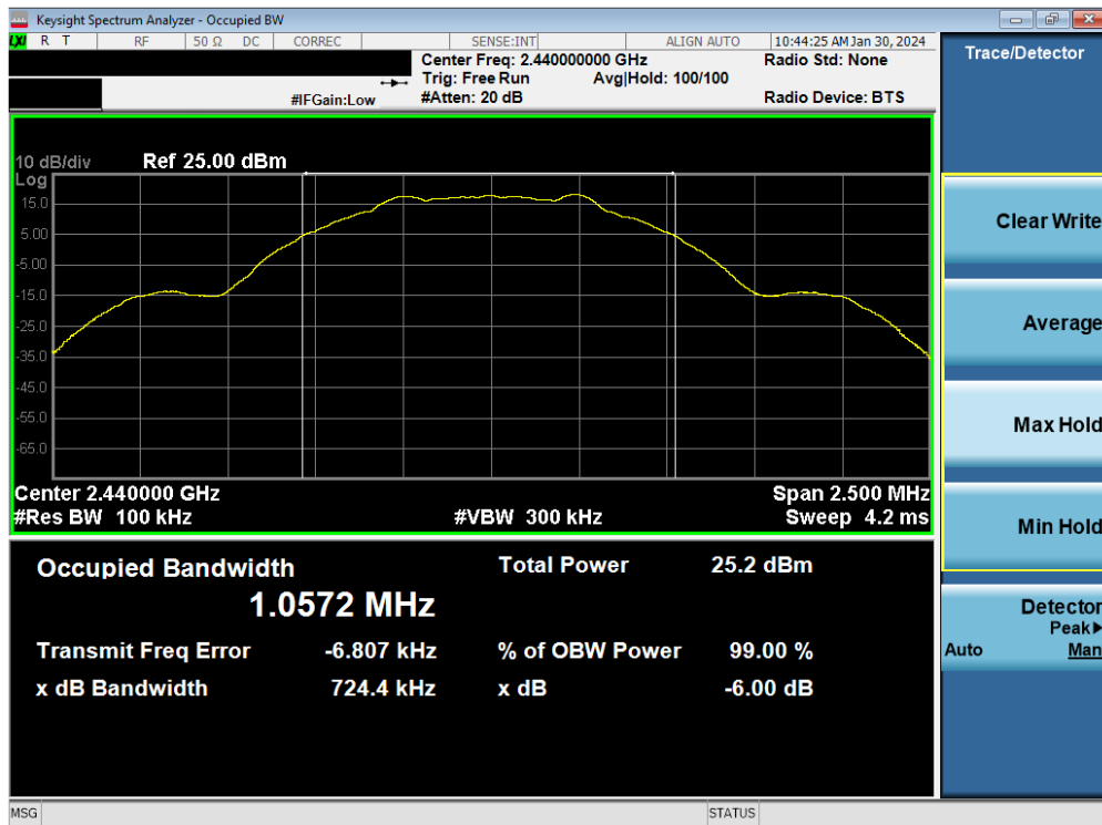
Plot 7-8. 6dB BW & 99% OBW Plot Antenna 2a (Bluetooth (LE), 1Mbps, ePA – Ch. 19)
