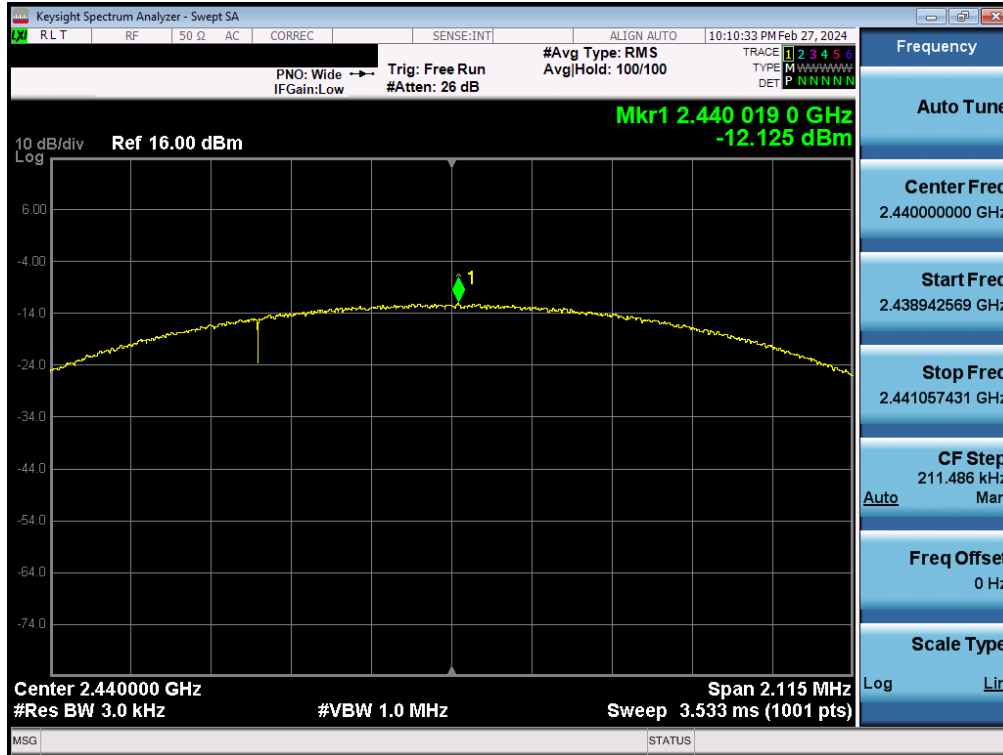
Plot 7-57. Power Spectral Density Plot Antenna 4a (Bluetooth (LE), 2Mbps, iPA – Ch. 19)
