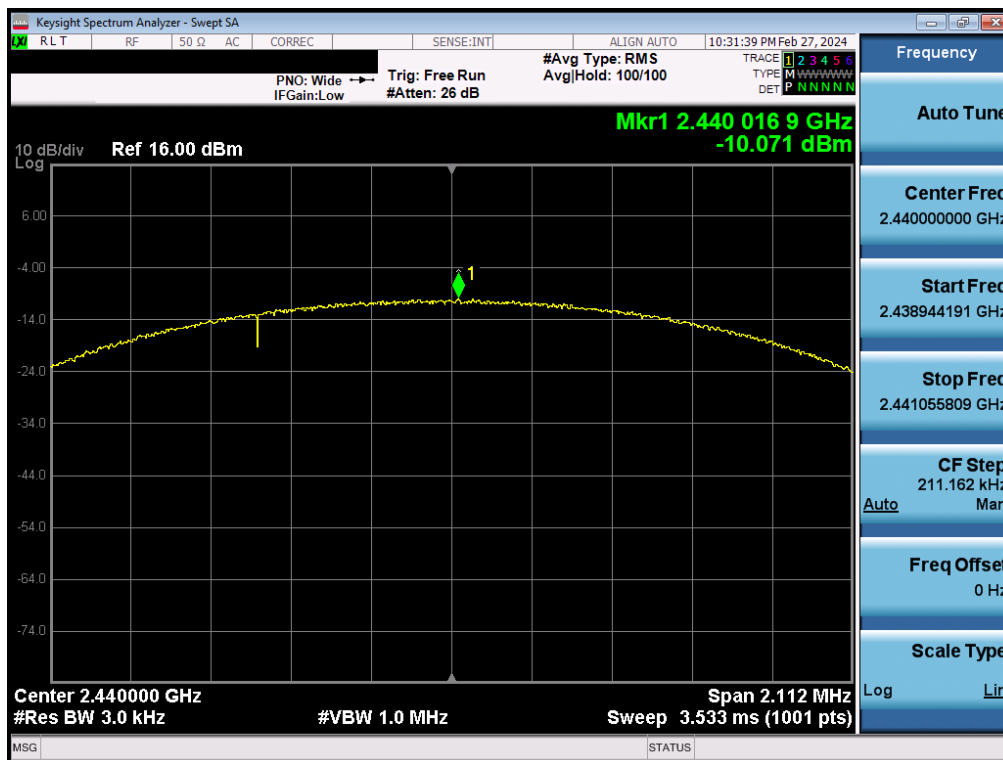
Plot 7-52. Power Spectral Density Plot Antenna 2a (Bluetooth (LE), 2Mbps, ePA – Ch. 19)
