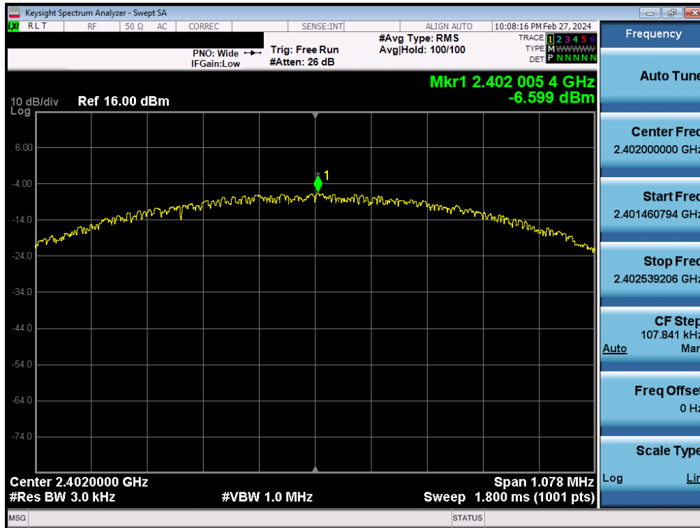
Plot 7-43. Power Spectral Density Plot Antenna 4a (Bluetooth (LE), 1Mbps, iPA – Ch. 0)
