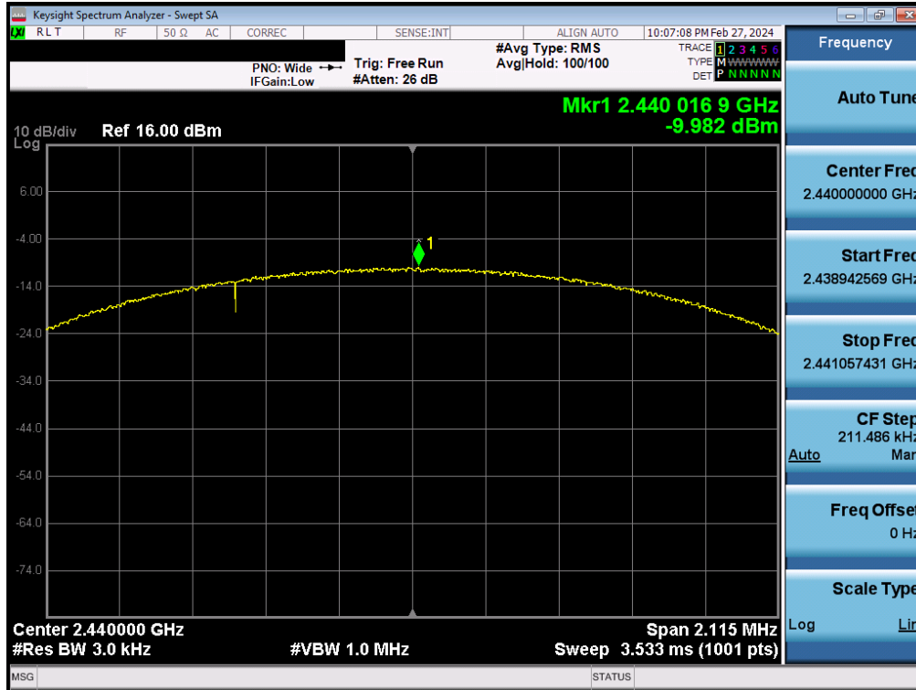
Plot 7-51. Power Spectral Density Plot Antenna 4a (Bluetooth (LE), 2Mbps, ePA – Ch. 19)
