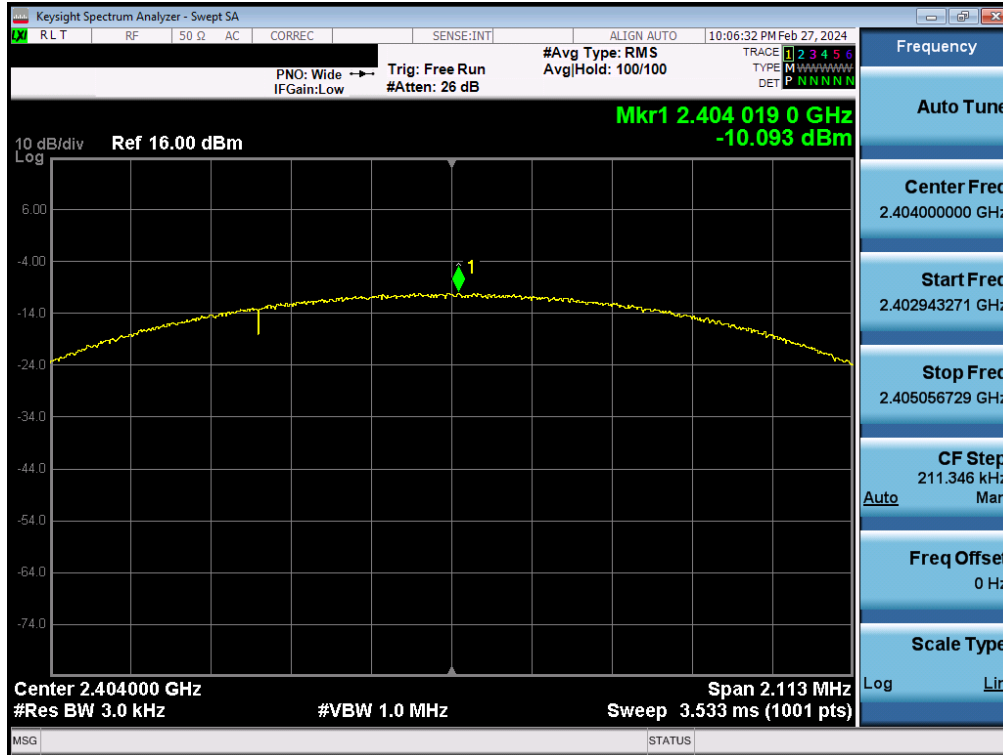
Plot 7-49. Power Spectral Density Plot Antenna 4a (Bluetooth (LE), 2Mbps, ePA – Ch. 1)
