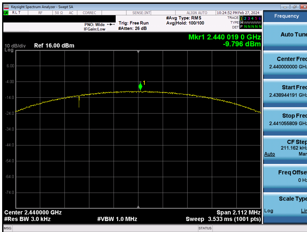
Plot 7-32. Power Spectral Density Plot Antenna 2a (Bluetooth (LE), 2Mbps, ePA – Ch. 19)
