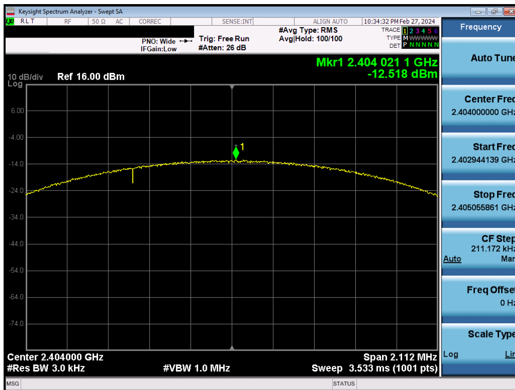
Plot 7-56. Power Spectral Density Plot Antenna 2a (Bluetooth (LE), 2Mbps, iPA – Ch. 1)
