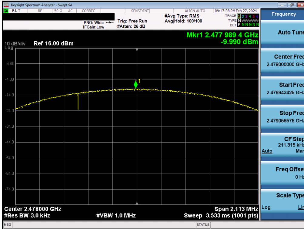
Plot 7-21. Power Spectral Density Plot Antenna 4a (Bluetooth (LE), 2Mbps, ePA – Ch. 38)
