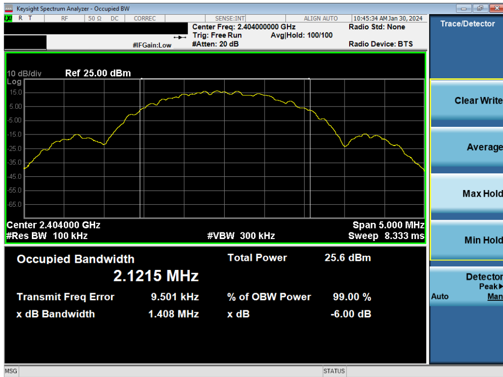
Plot 7-10. 6dB BW & 99% OBW Plot Antenna 2a (Bluetooth (LE), 2Mbps, ePA – Ch. 1)
