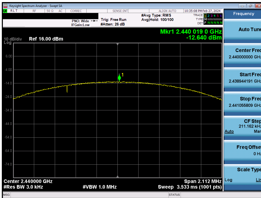
Plot 7-58. Power Spectral Density Plot Antenna 2a (Bluetooth (LE), 2Mbps, iPA – Ch. 19)
