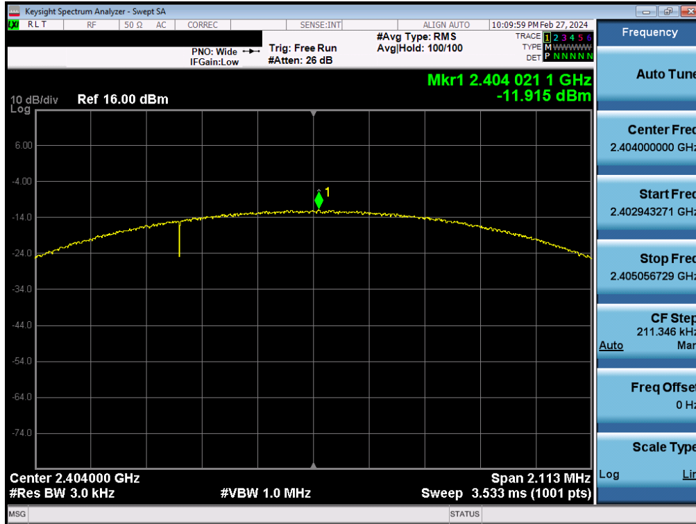
Plot 7-55. Power Spectral Density Plot Antenna 4a (Bluetooth (LE), 2Mbps, iPA – Ch. 1)
