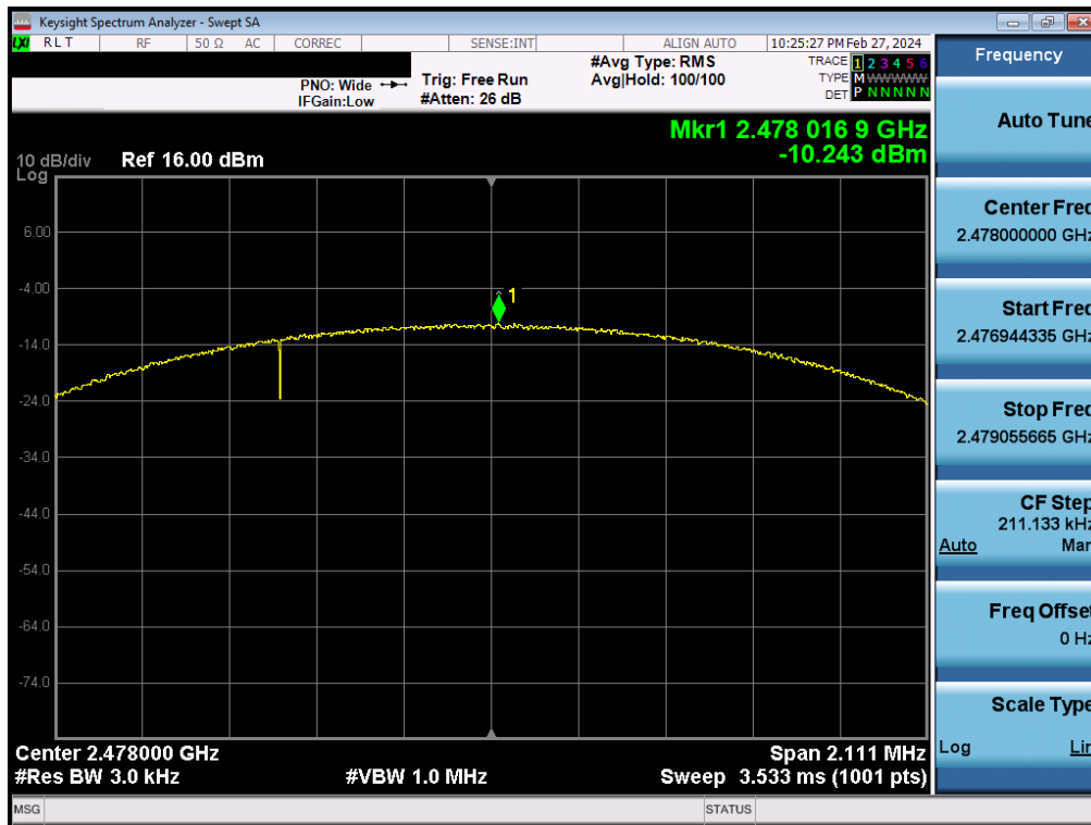
Plot 7-33. Power Spectral Density Plot Antenna 2a (Bluetooth (LE), 2Mbps, ePA – Ch. 38)
