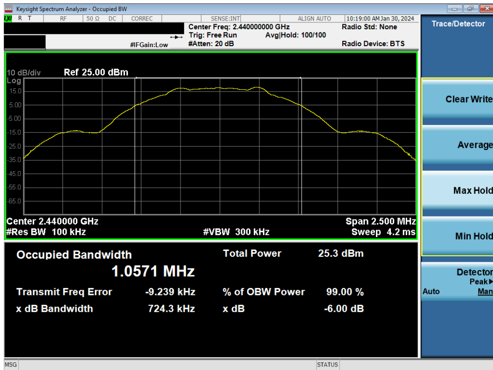
Plot 7-2. 6dB BW & 99% OBW Plot Antenna 4a (Bluetooth (LE), 1Mbps, ePA – Ch. 19)
