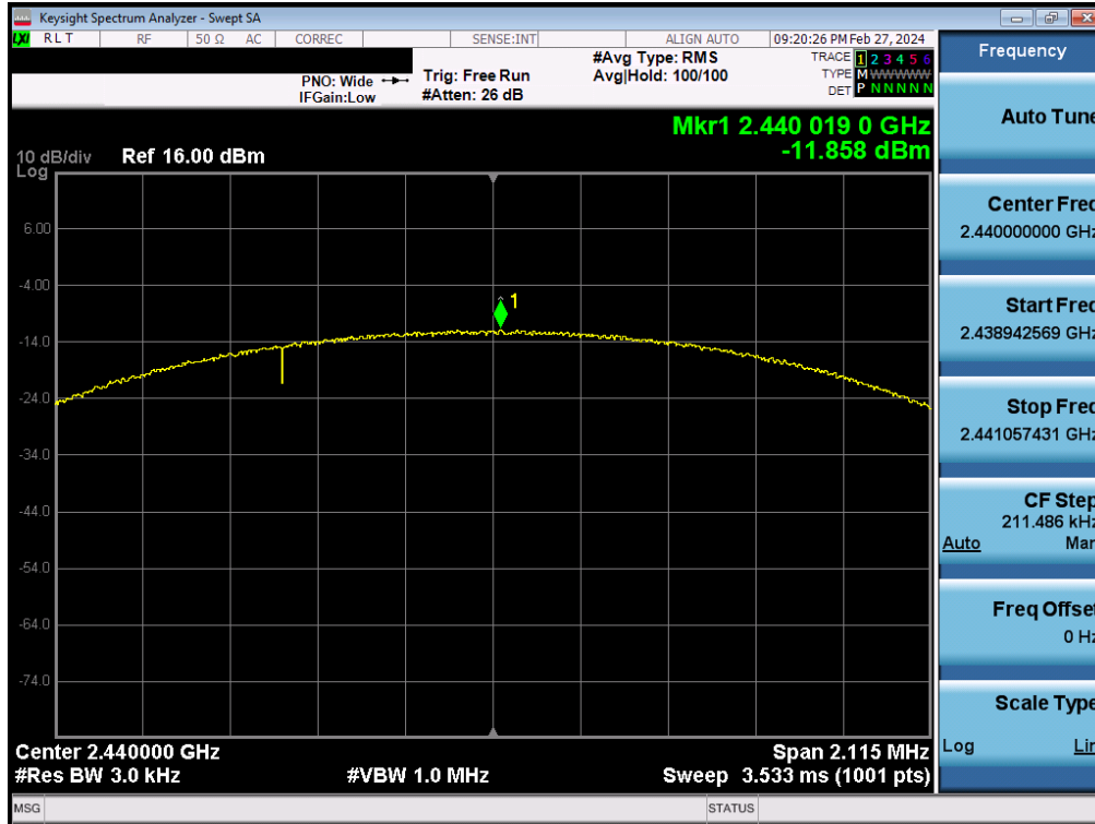
Plot 7-23. Power Spectral Density Plot Antenna 4a (Bluetooth (LE), 2Mbps, iPA – Ch. 19)
