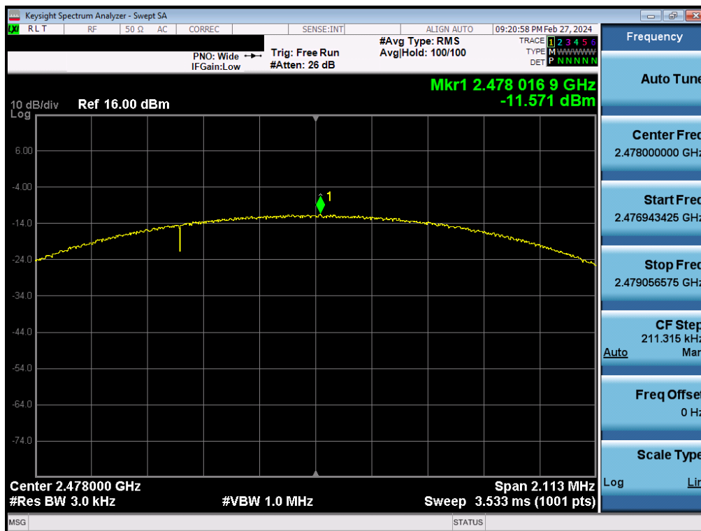
Plot 7-24. Power Spectral Density Plot Antenna 4a (Bluetooth (LE), 2Mbps, iPA – Ch. 38)
