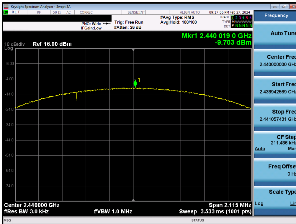
Plot 7-20. Power Spectral Density Plot Antenna 4a (Bluetooth (LE), 2Mbps, ePA – Ch. 19)
