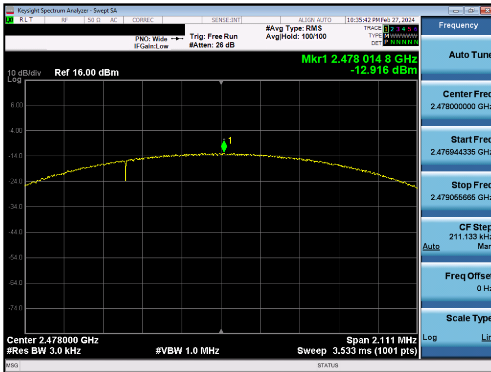
Plot 7-60. Power Spectral Density Plot Antenna 2a (Bluetooth (LE), 2Mbps, iPA – Ch. 38)
