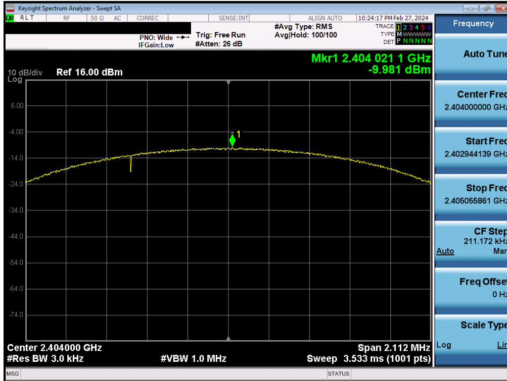
Plot 7-31. Power Spectral Density Plot Antenna 2a (Bluetooth (LE), 2Mbps, ePA – Ch. 1)
