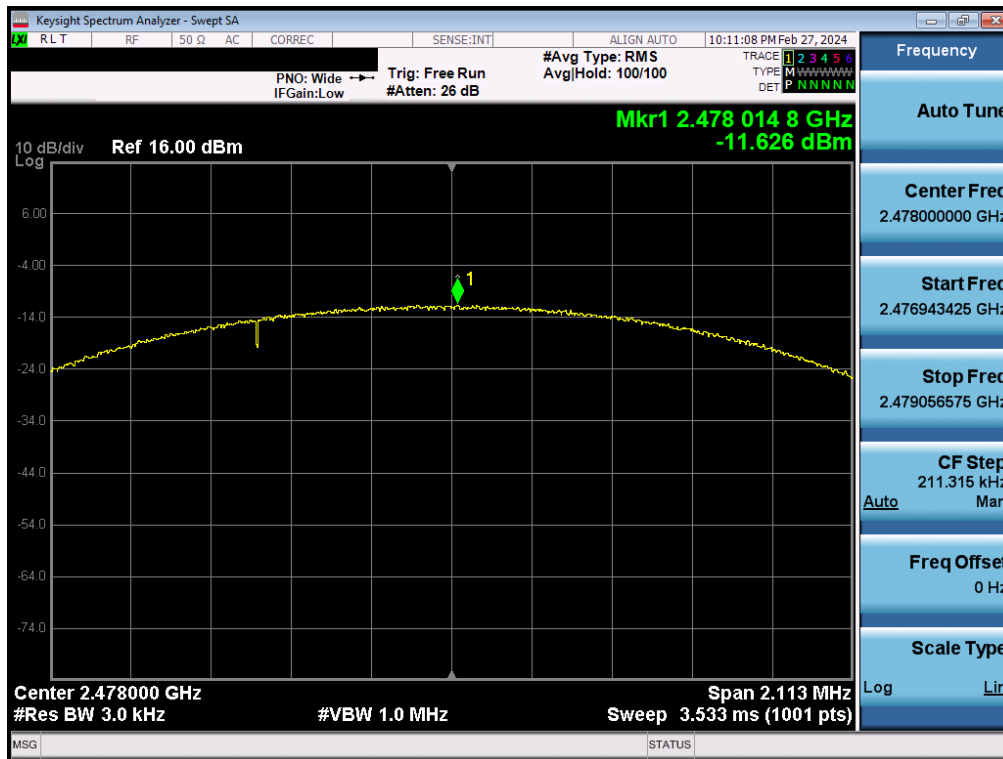
Plot 7-59. Power Spectral Density Plot Antenna 4a (Bluetooth (LE), 2Mbps, iPA – Ch. 38)
