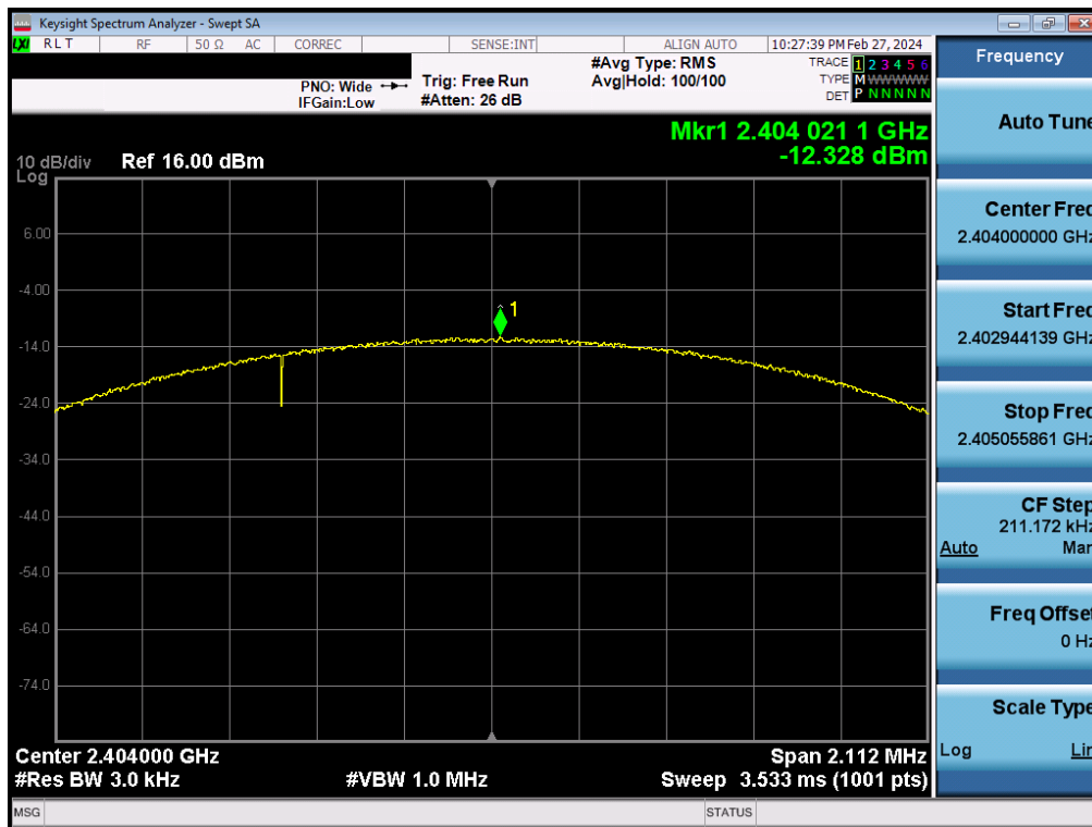
Plot 7-34. Power Spectral Density Plot Antenna 2a (Bluetooth (LE), 2Mbps, iPA – Ch. 1)
