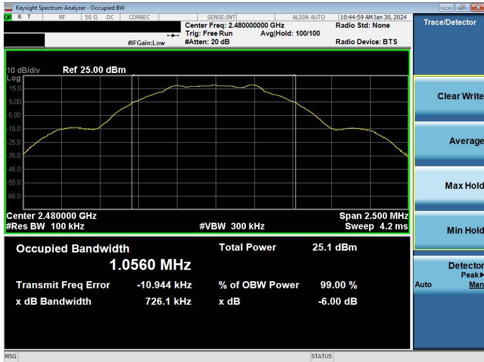
Plot 7-9. 6dB BW & 99% OBW Plot Antenna 2a (Bluetooth (LE), 1Mbps, ePA – Ch. 39)
