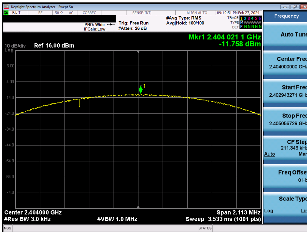
Plot 7-22. Power Spectral Density Plot Antenna 4a (Bluetooth (LE), 2Mbps, iPA – Ch. 1)
