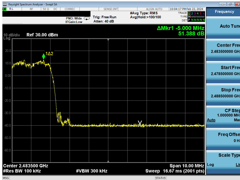
Plot 7-28. Band Edge Plot Antenna 2a (Bluetooth with Hopping Enabled, 8DPSK, ePA)
