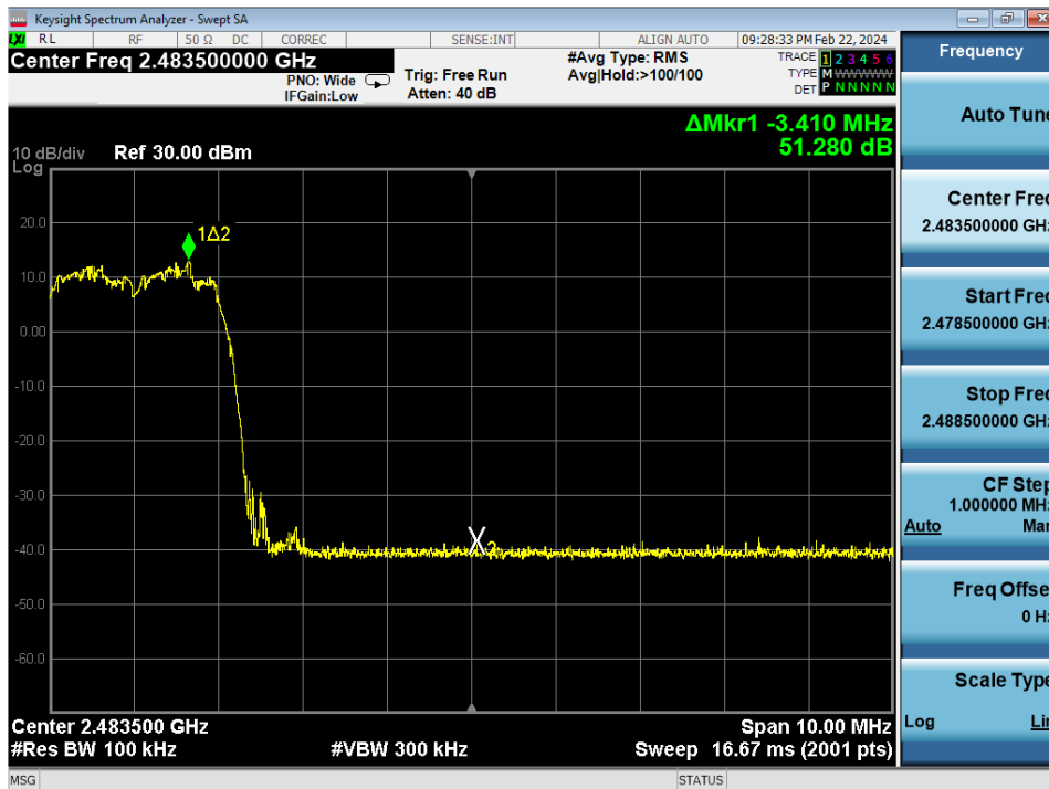
Plot 7-20. Band Edge Plot Antenna 4a (Bluetooth with Hopping Enabled, 8DPSK, ePA)
