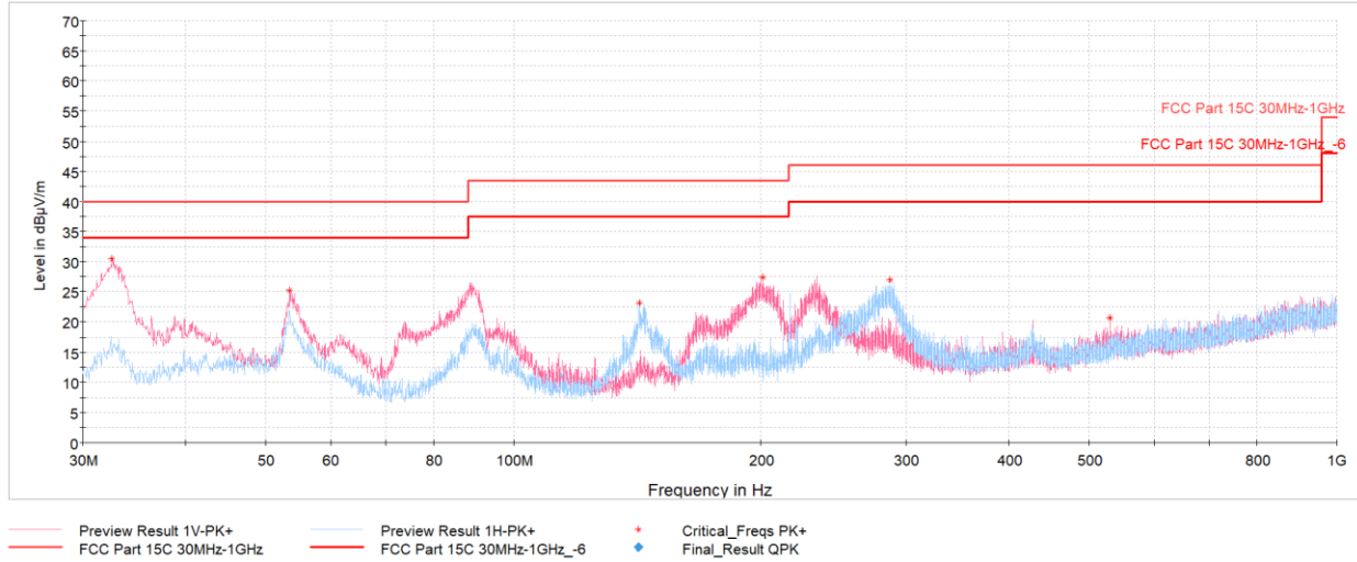
Plot 7-83. Radiated Spurious Emissions Below 1GHz TxBF (GFSK ePA – Ch.39, with Laptop)
