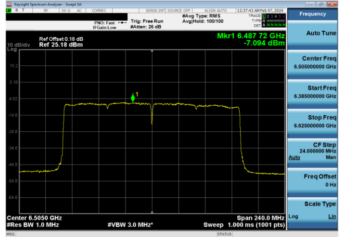
Plot 7-224. Power Spectral Density Plot LPI Antenna WF8 (160MHz 802.11ax (UNII Band 6) - Ch. 111, MCS2)
