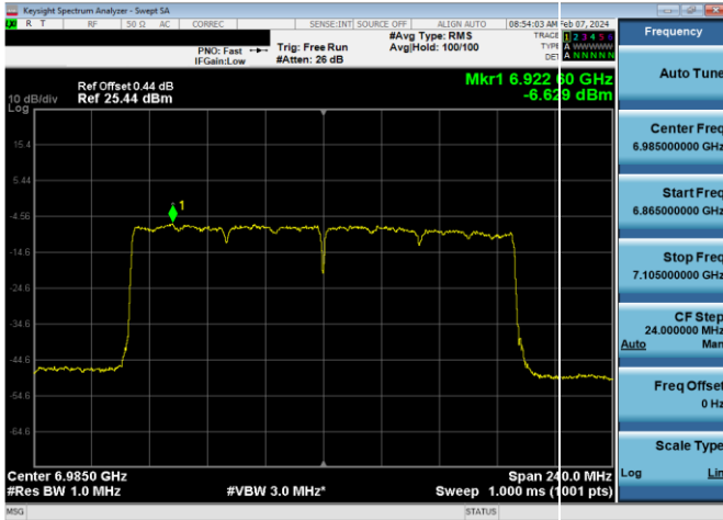
Plot 7-274. Power Spectral Density Plot LPI Antenna WF8 (160MHz 802.11ax (UNII Band 8) - Ch. 207, MCS11)
