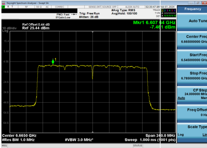
Plot 7-269. Power Spectral Density Plot LPI Antenna WF8 (160MHz 802.11ax (UNII Band 7) – Ch. 143, MCS11)
