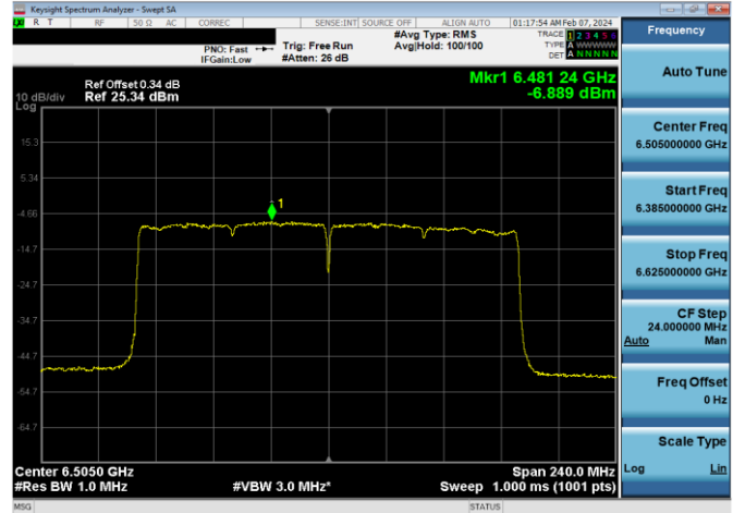
Plot 7-244. Power Spectral Density Plot LPI Antenna WF8 (160MHz 802.11ax (UNII Band 6) – Ch. 111, MCS4)
