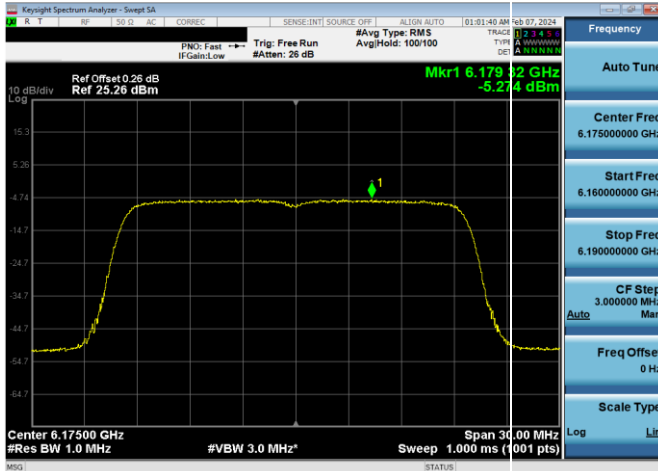
Plot 7-236. Power Spectral Density Plot LPI Antenna WF8 (20MHz 802.11ax (UNII Band 5) - Ch. 45, MCS4)
