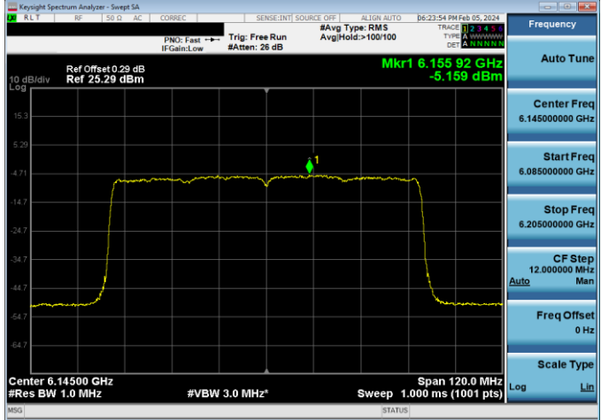
Plot 7-220. Power Spectral Density Plot LPI Antenna WF5B (80MHz 802.11ax (UNII Band 5) - Ch. 39, MCS11)
