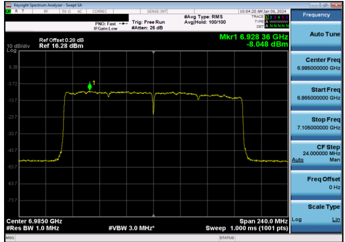
Plot 7-184. Power Spectral Density Plot LPI Antenna 5T LPI (160MHz 802.11ax (UNII Band 8) – Ch. 207, MCS4)
