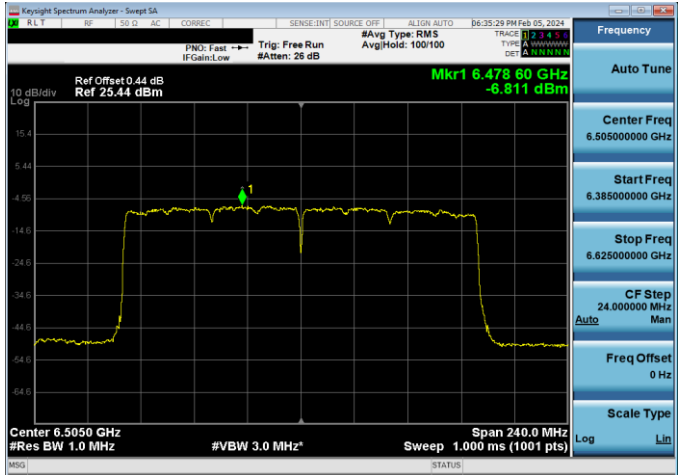
Plot 7-226. Power Spectral Density Plot LPI Antenna WF5B (160MHz 802.11ax (UNII Band 6) - Ch. 111, MCS11)
