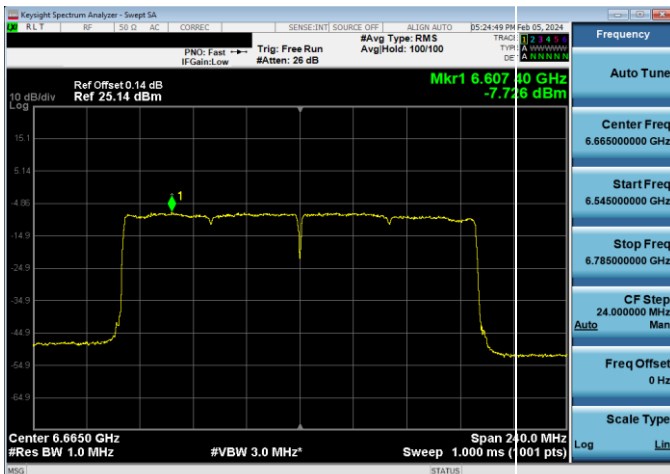
Plot 7-195. Power Spectral Density Plot LPI Antenna WF5B (160MHz 802.11ax (UNII Band 7) - Ch. 143, MCS2)
