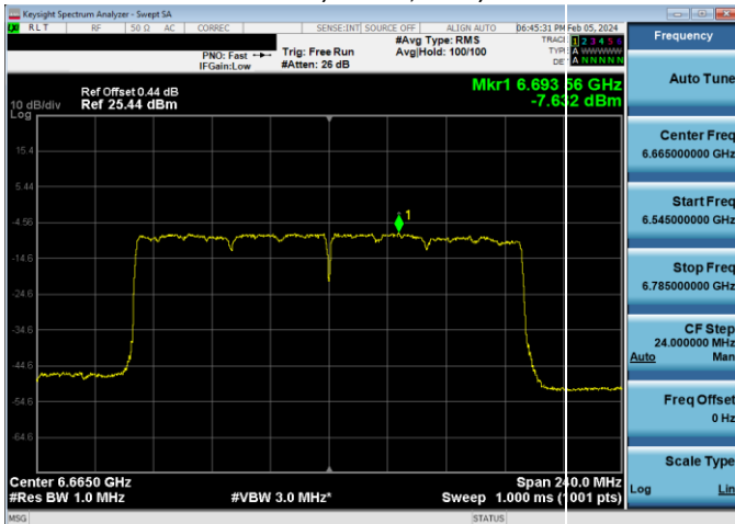
Plot 7-231. Power Spectral Density Plot LPI Antenna WF5B (160MHz 802.11ax (UNII Band 7) - Ch. 143, MCS11)
