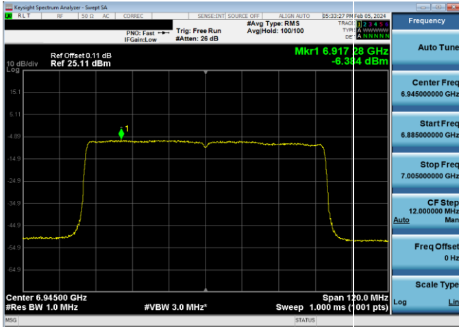
Plot 7-199. Power Spectral Density Plot LPI Antenna WF5B (80MHz 802.11ax (UNII Band 8) – Ch. 199, MCS2)
