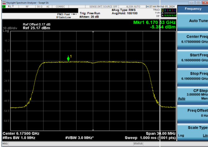
Plot 7-182. Power Spectral Density Plot LPI Antenna WF5B (20MHz 802.11ax (UNII Band 5) - Ch. 45, MCS2)
