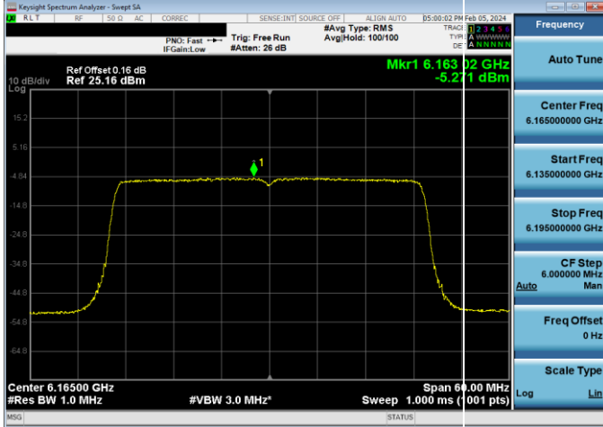
Plot 7-183. Power Spectral Density Plot LPI Antenna WF5B (40MHz 802.11ax (UNII Band 5) - Ch. 43, MCS2)
