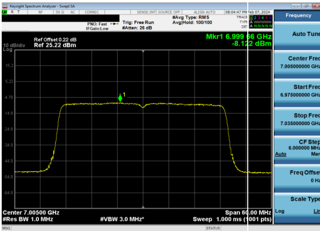
Plot 7-847. LPI Power Spectral Density Plot SDM Diversity Antenna WF8 (40MHz 802.11ax RU484 (UNII Band 8) – Ch. 211)
