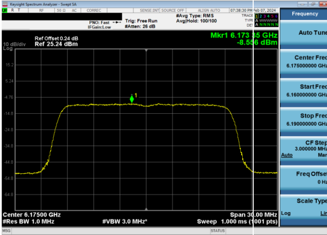
Plot 7-743. LPI Power Spectral Density Plot SDM Diversity Antenna WF8 (20MHz 802.11ax RU242 (UNII Band 5) – Ch. 45)
